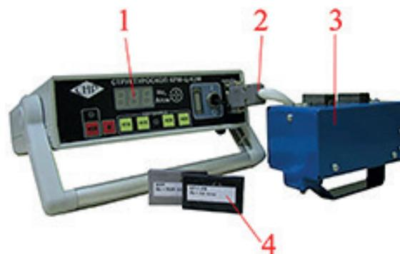
Fig. 1 The exterior of the KRM-CK-2M device: 1 – measuring block; 2 – connecting cable; 3 – transformer; 4 – control samples
