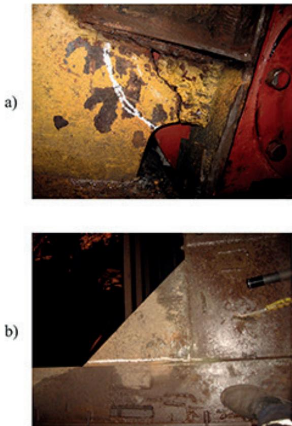
**Fig. 7** Defect cracks (indicated by white color) in the bearing box zone (a) and the connection zone of the end and main beams (b) of the crane
