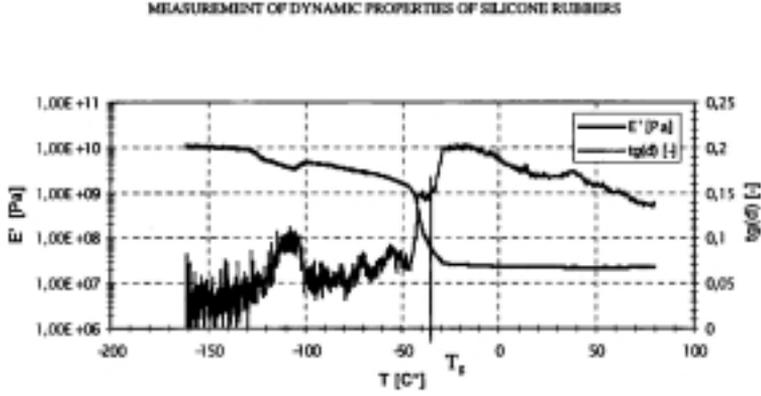
Fig. 4. The thermomechanical curves of 40 Sh P silicone rubber
