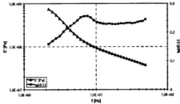
Fig. 5. The storage modulus and the loss rate of 30 A silicone rubber depending on frequency at  $T_0 = T_g$
