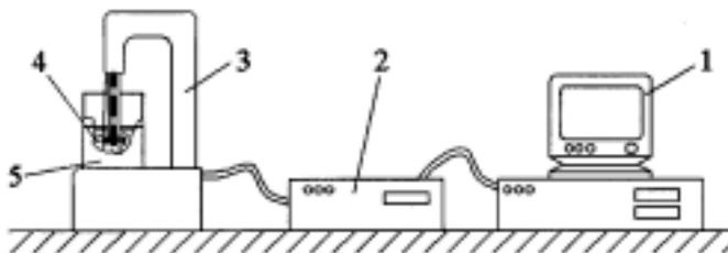
*Fig. 1.* The equipment of the Dynamic Mechanical Analysis
