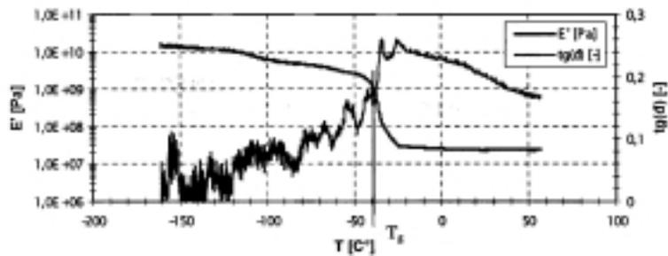
*Fig. 3.* The thermomechanical curves of 30 Sh A silicone rubber
