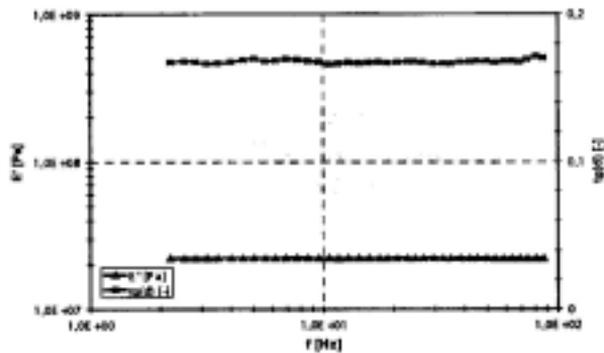
Fig. 8. The storage modulus and the loss rate of 40 P silicone rubber depending on frequency at  $T_0 = 20\text{ }^\circ\text{C}$
