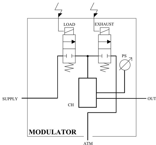
*Fig. 1.* Functional representation of the electro-pneumatic modulator
