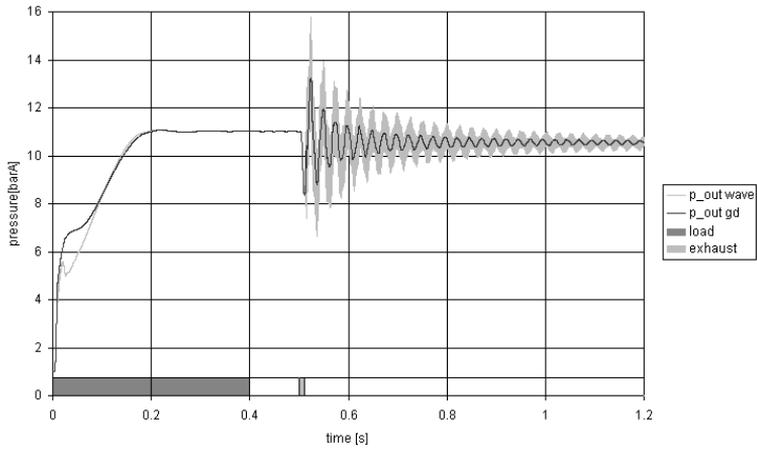
*Fig. 6.* Modulator chamber pressure, Test case 2
