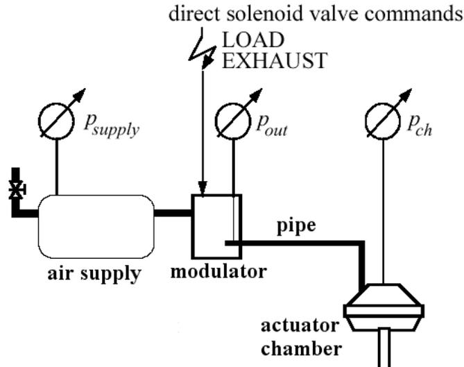
*Fig. 2.* Scheme of case study set-up
