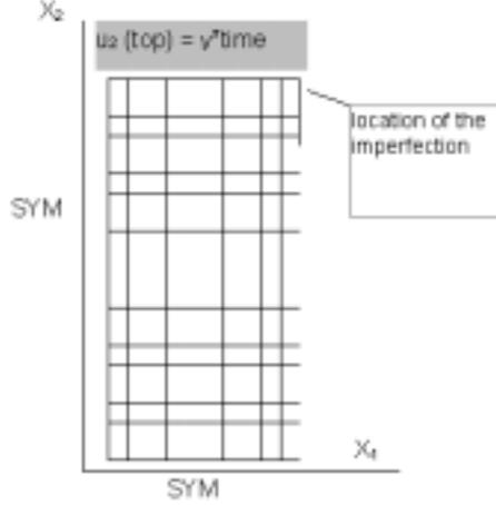
*Fig. 1.* Boundary and loading conditions
