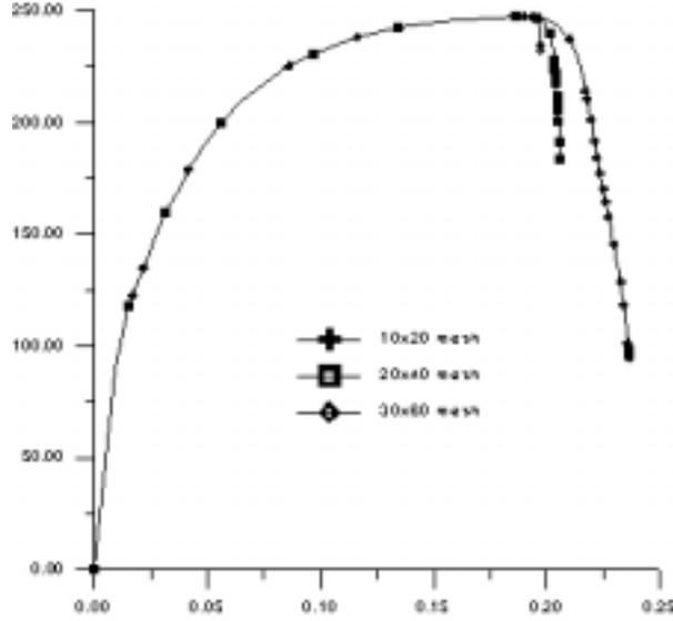
Fig. 2. Mesh dependence of the load-displacement curves for damageable material without viscosity
