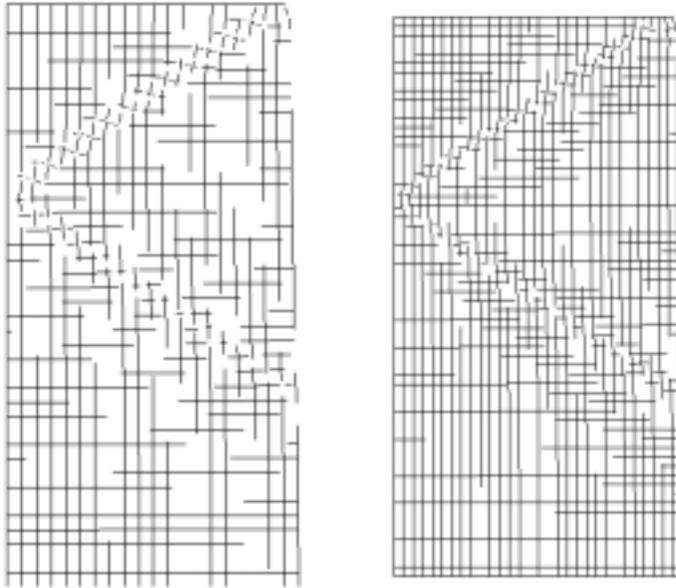
Fig. 3. Simulation of shear bands with a coarse and a fine mesh
