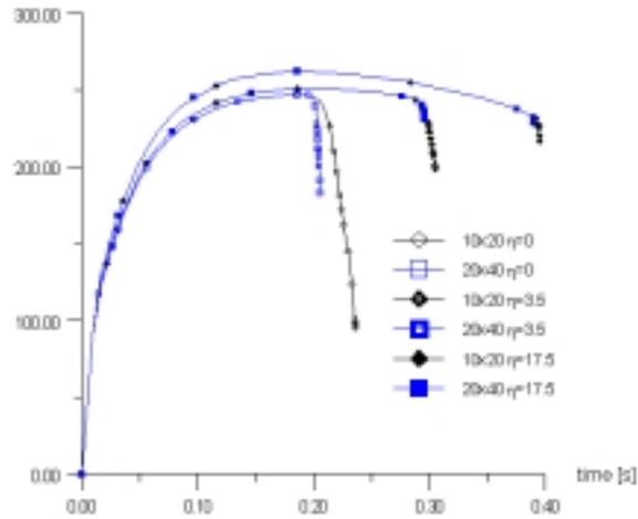
Fig. 5. Mesh dependence of the load-displacement curves for several values of a viscosity parameter ( $\eta \in \{0; 3.5; 17.5\}$ )
