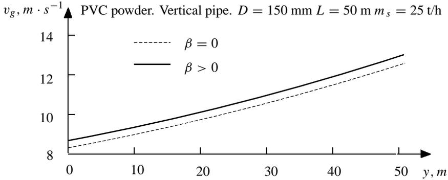
Fig. 6. Gas velocity along the pipe length
