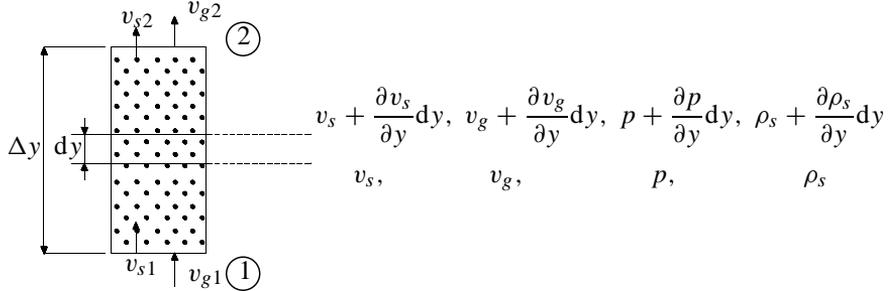
Fig. 1. Elementary pipe section cut from a vertical pipeline
