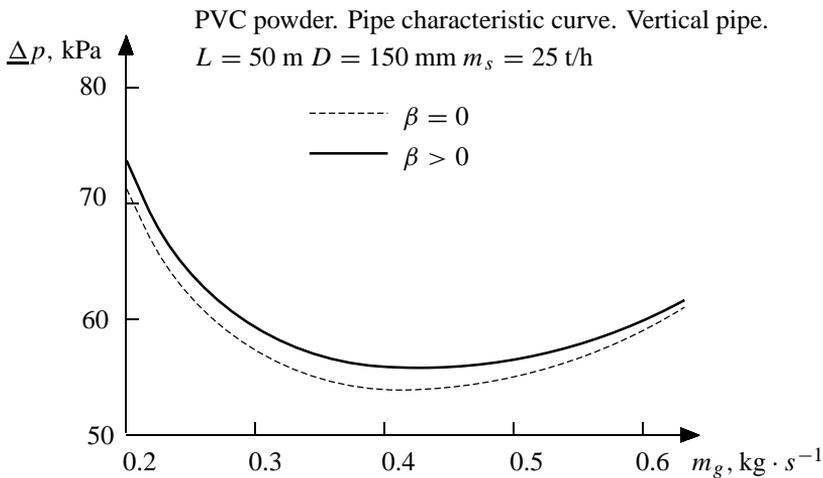
Fig. 11. Pressure drop in the conveying pipe as function of the gas mass flow
