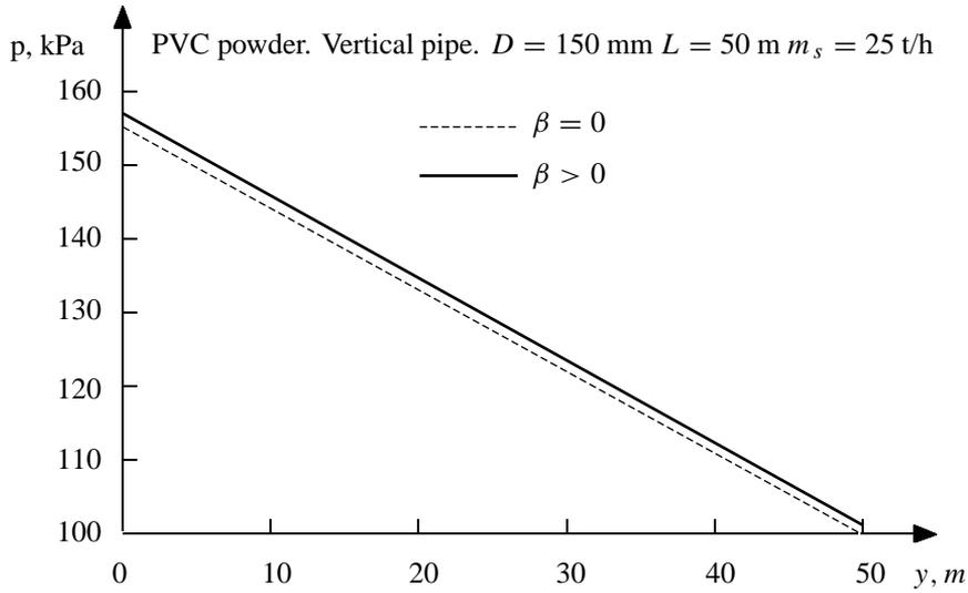
Fig. 2. Calculated pressure as function of the pipe length
