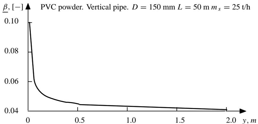
Fig. 9. Change of ' $\beta$ ' as function of the pipe length in the initial section of the pipe
