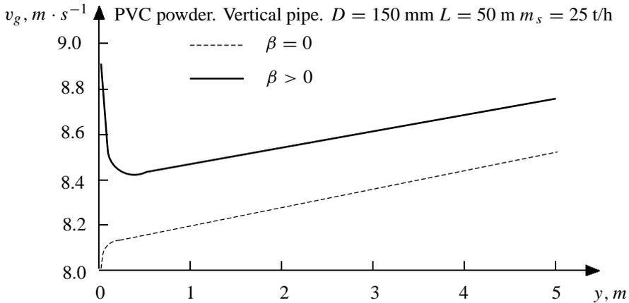
Fig. 7. Gas velocity along the pipe length in the initial section of the pipe
