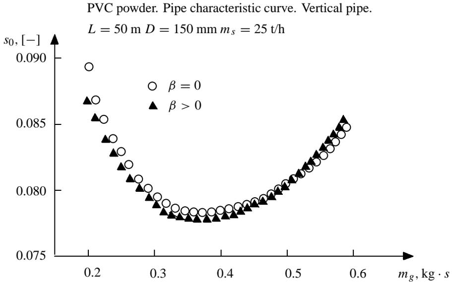
Fig. 12. Slip at the pipe end as function of the gas mass flow
