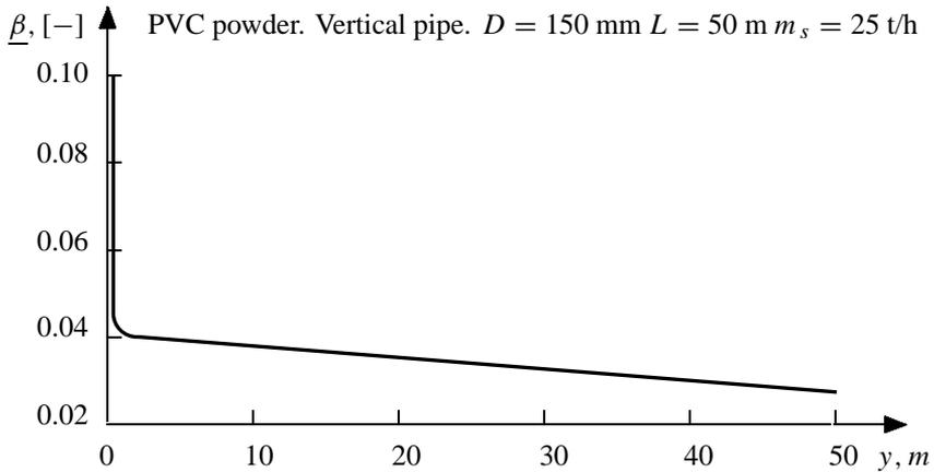
Fig. 8. Change of ' $\beta$ ' as function of the pipe length
