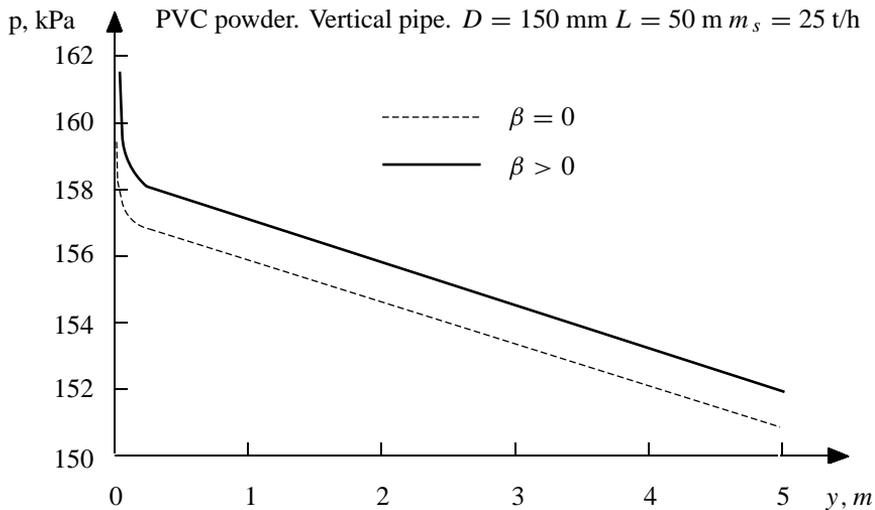
Fig. 3. Calculated pressure as function of the pipe length in the initial section of the pipe
