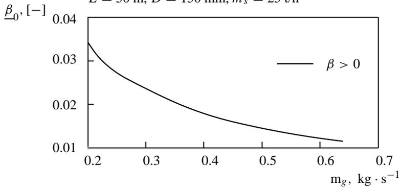
Fig. 14. Change of ' $\beta_0$ ' as function of the gas mass flow
