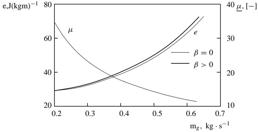
Fig. 13. Specific energy consumption and mixing ratio as function of the gas mass flow
