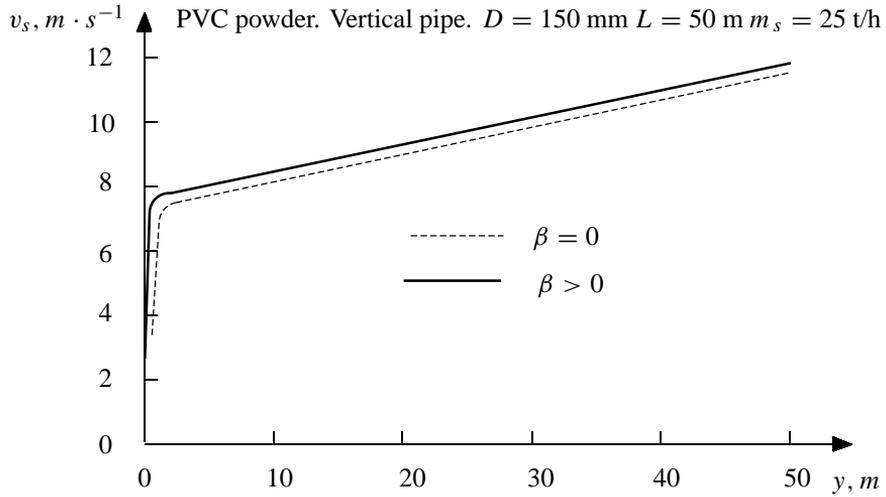
Fig. 4. Material velocity as function of the pipe length
