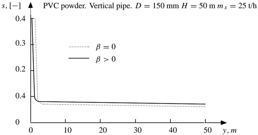
Fig. 10. Change of slip as function of the pipe length
