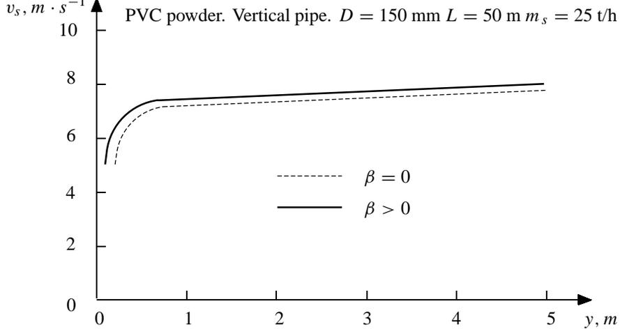
Fig. 5. Material velocity as function of the pipe length in the initial section of the pipe
