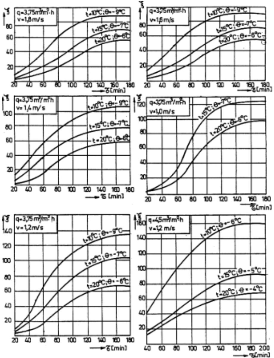
Fig. 2. The variation of aerodynamic resistance coefficient ( $\xi$ ) for the simple ice curtain system
