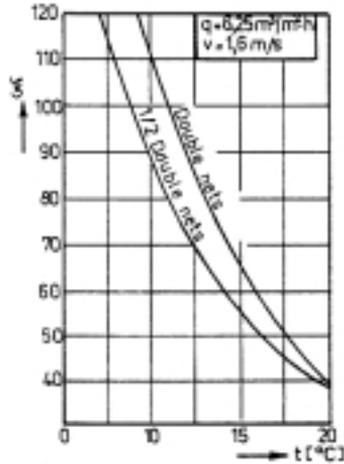
Fig. 4. The correlation between the aerodynamic resistance coefficient and the water temperature for cases A) and B) of the self-protecting system
