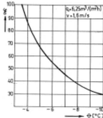
Fig. 5. The correlation between the resistance coefficient and air temperature in case A).
