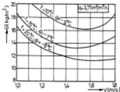
Fig. 3. The correlation of specific ice load of the self-protecting curtain
