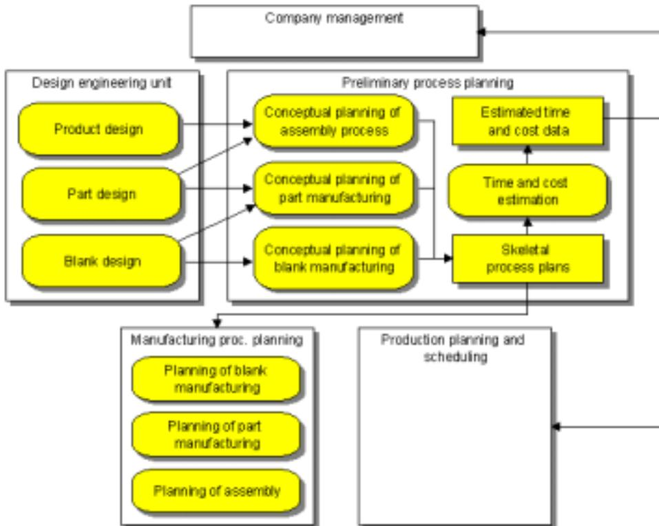
Fig. 8. Skeletal process planning and time and cost estimation
