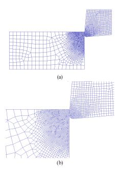
Fig. 2 (a) Meshed Geometry, (b) Local refinement at the contact
