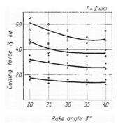
**Fig. 7** Relations for rake angle according to [22]
