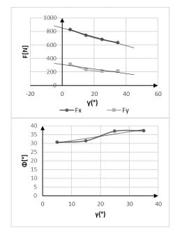
Fig. 6 Relations for rake angle
