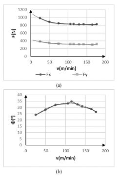
**Fig. 13** (a) Force relations for cutting velocity (b) Shear angle relation for cutting velocity
