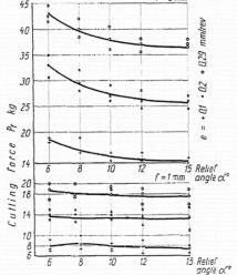
Fig. 5 Relations for relief angle according to [22]
