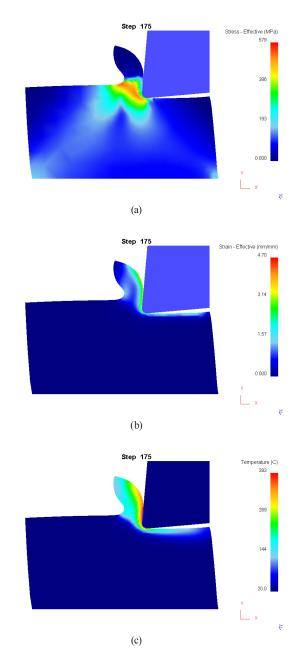
Fig. 3 (a) Stress distribution on examined geometry nr.0,(b) Strain distribution on examined geometry nr.0,(c) Temperature distribution on examined geometry nr.0
