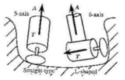
Fig. 4. Necessity of 6-axis control [1]
