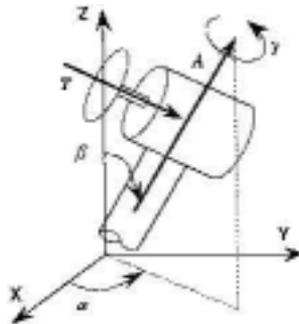
*Fig. 5.* Tool attitude in the robot coordinate system [1]
