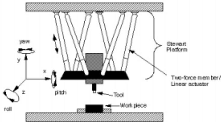
Fig. 1. Schematic of a hexapod six-axis machining center
