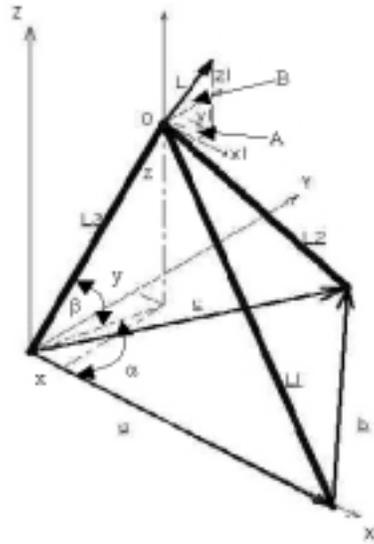
Fig. 5. Schematic model of the tripod kinematics
