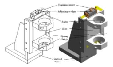
Fig. 2. The CAD model of the fixture
