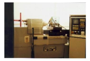
Fig. 1. The ULTRATURN UP1 high precision lathe
