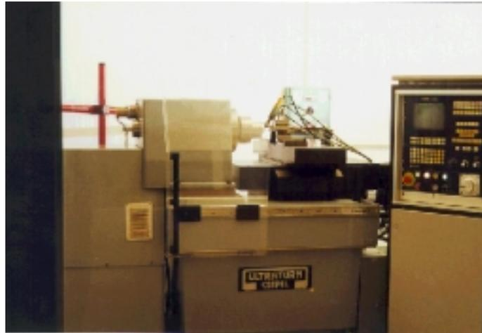
*Fig. 1.* The ULTRATURN UP1 high precision lathe
