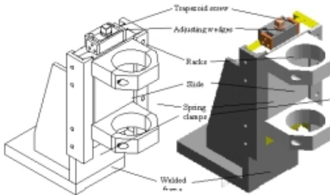
Fig. 2. The CAD model of the fixture
