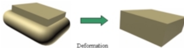
Fig. 2. The deformation of undercuts in the foam during demoulding
