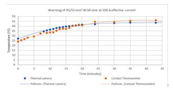
Fig. 1 Measurement - Warming of 95/55 mm<sup>2</sup> ACSR wire at 200 A effective current
