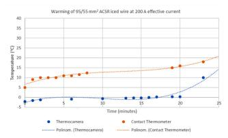
Fig. 7 Warming of 95/55 mm<sup>2</sup> ACSR iced wire at 200 A effective current
