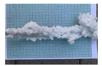
Fig. 4 Ripped iced wire
