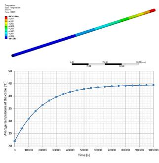
Fig. 9 The final temperature and the warming up procedure of the cable after current heating during the FEA
