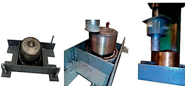
Fig. 14 General view of the auxiliary device SRP-1 for the study of the stamping by rolling process
