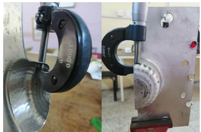
Fig. 10 Method of the measurement of thickness distribution
