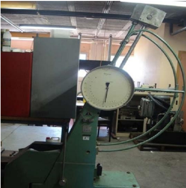
Fig. 4 Pendulum for Charpy test
