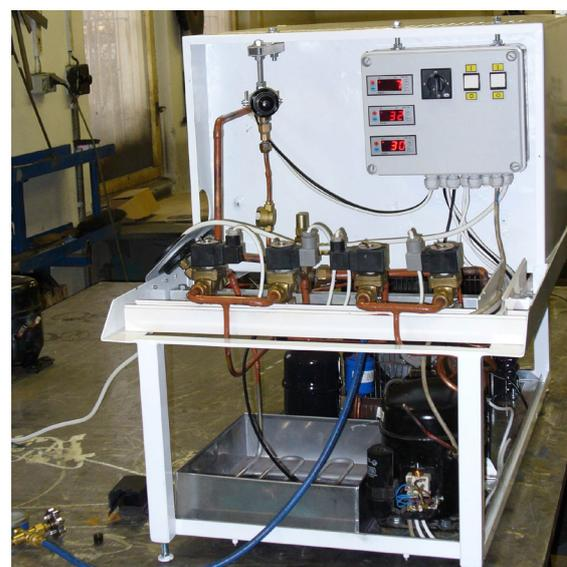
Fig. 3 The experimental cooling circuit equipped with a desuperheater, set up for the study
