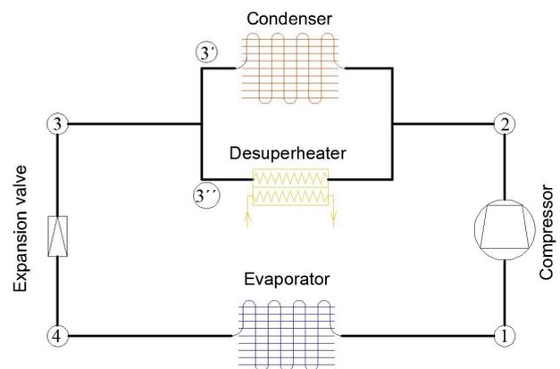
Fig. 1 Schematic of a cooling circuit with a parallel connected desuperheater, including operating points
