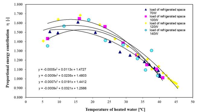
Fig. 11 Relationship between  $\eta$  and temperature of heated water for the parallel connected condenser and desuperheater
