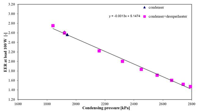
Fig. 6 Relationship between EER and condensing pressure, at a cooling load of 100 watts
