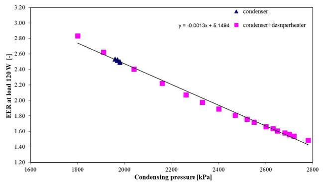
Fig. 7 Relationship between EER and condensing pressure, at a cooling load of 120 watts
