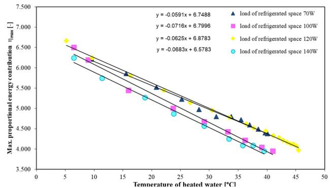
Fig. 10 Relationship between  $\eta_{max}$  and temperature of heated water for the parallel connected condenser and desuperheater
