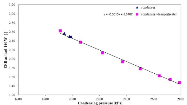
Fig. 8 Relationship between EER and condensing pressure, at a cooling load of 140 watts
