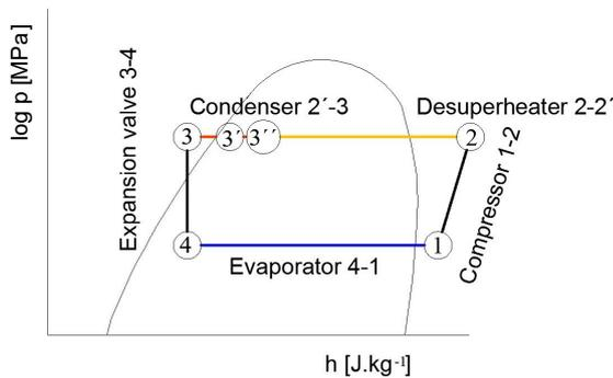
Fig. 2 Schematic of the principle of a cooling circuit operating with a desuperheater in a p-h diagram
