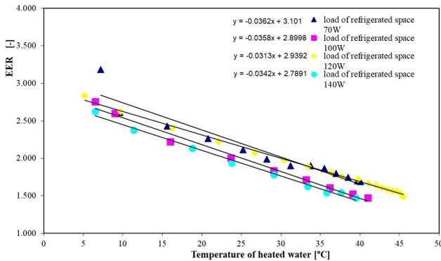
Fig. 9 Relationship between EER and temperature of heated water for the parallel connected condenser and desuperheater
