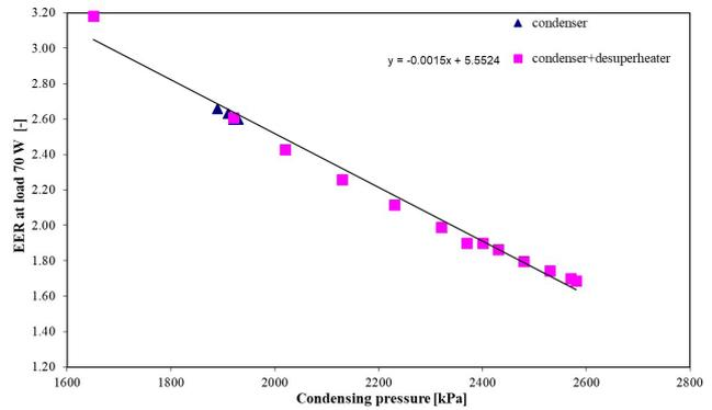
Fig. 5 Relationship between EER and condensing pressure, at a cooling load of 70 watts
