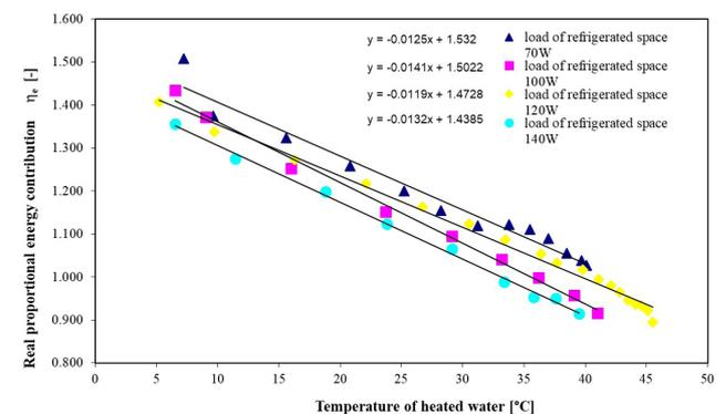
Fig. 12 Relationship between  $\eta_e$  and temperature of heated water for the condenser only
