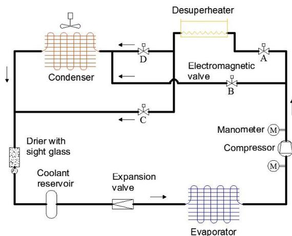
Fig. 4 Diagram of test circuit with marking of control valves
