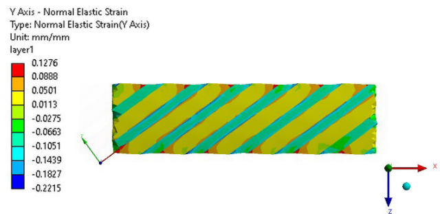
Fig. 14 Normal strain in material direction 2 in layer 1 between x = -4 mm and x = 4 mm
