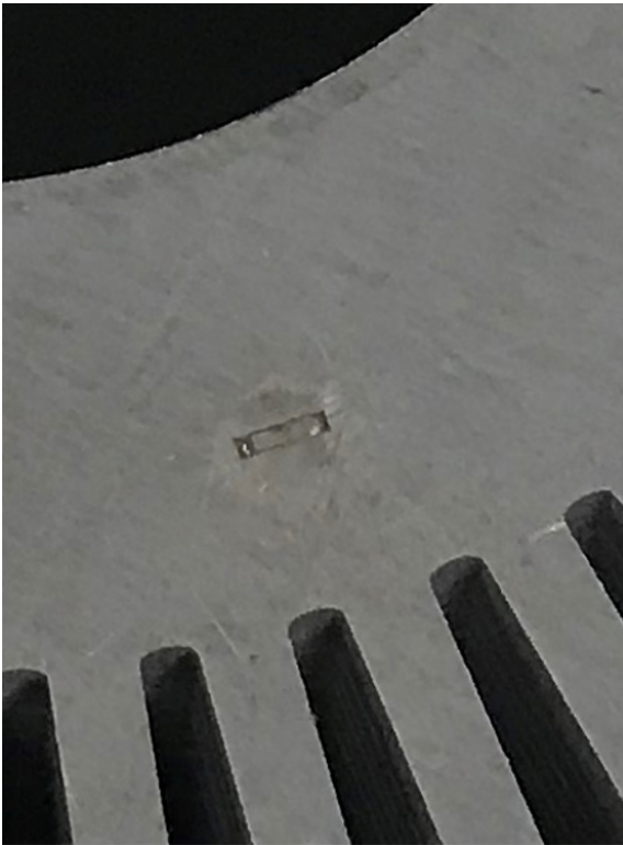
Fig. 4 Laminate stack joined using stamping
