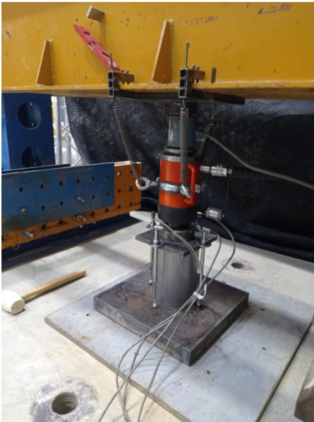
Fig. 7 Image of an axial compression loading test
