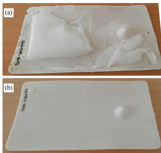
Fig. 5 Samples with low (a) and good surface adhesion (b)
