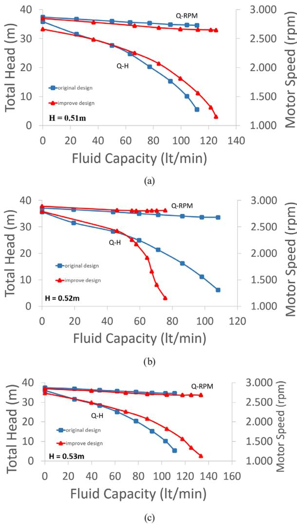
**Fig. 4** Performance graphs comparing the existing and modified impeller designs by various discharge head (a) 0.51 m; (b) 0.52 m, and (c) 0.53 m
