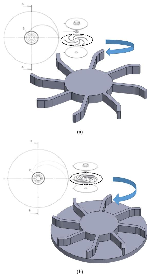
**Fig. 1** (a) Existing model and (b) modified model of a centrifugal pump impeller
