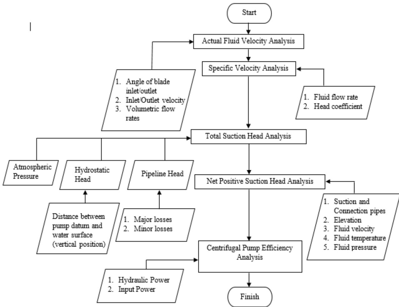
Fig. 3 Flowchart analysis scheme of centrifugal impeller design
