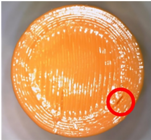
Fig. 8 Printing failure, Note: 0.4 mm layer thickness, vertical orientation
