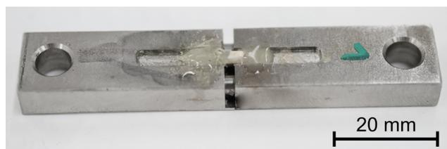
**Fig. 3** Jig used for the microtensile bond strength tests
