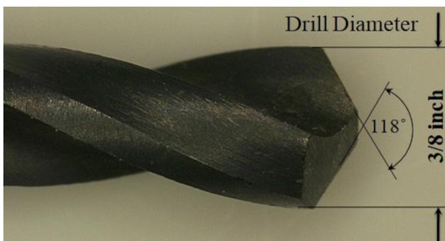
**Fig. 2** Uncoated high-speed steel twist drill used for drilling A356 blocks
