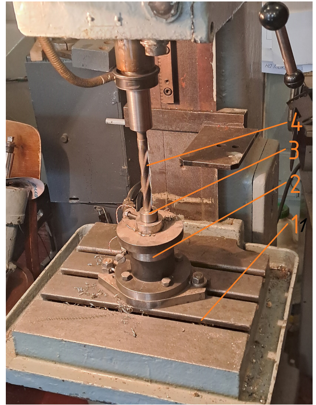
Fig. 2 (a) Scheme of the installation and (b) photo of the machining area: 1 - machine table; 2 - dynamometer; 3 - blank; 4 - tool; 5 - power supply; 6 - strain gauge station; 7 - recording device
