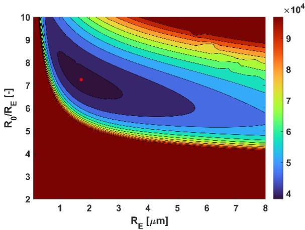
**Fig. 2** Energy intensity of hydrogen production (in terms of MJ/kg) at 1 bar and 25 °C as a function of the bubble radius and expansion ratio. The dot represents the optimum parameter combination.
