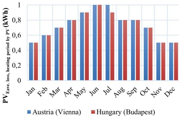
Fig. 3 Daily loss of energy in the electric water heating system during the period when water is heated by photovoltaic power
