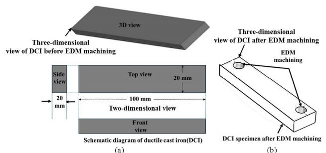
**Fig. 3** Schematic 2D and 3D views of work specimen with detailed specifications: (a) 2D views; and (b) 3D view showing holes at both ends after EDM machining
