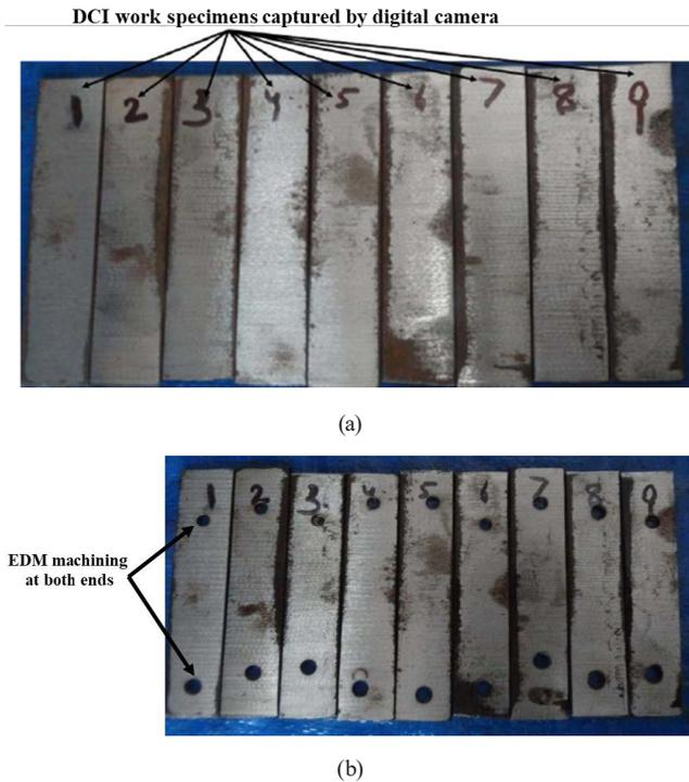
**Fig. 5** Photographs of the actual work specimens used in this study, captured by a digital camera: (a) before machining; and (b) after machining
