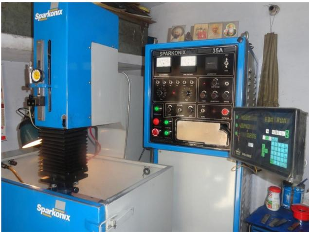
**Fig. 1** Electrical discharge machine used for machining ductile cast iron in this study
