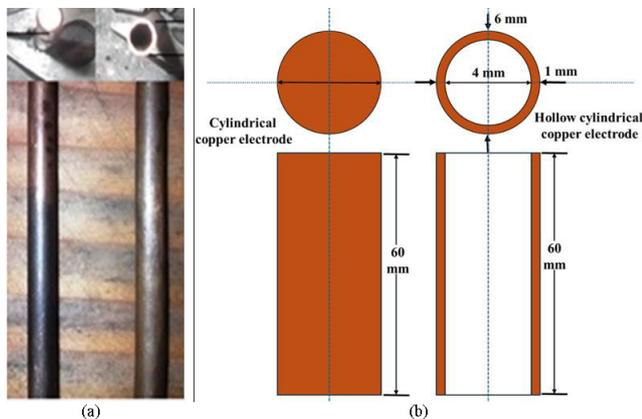
**Fig. 2** Cylindrical copper electrode used for machining DCI by EDM: (a) Pictorial 3-D view of both electrodes; and (b) schematic two-dimensional view of copper electrodes with detailed specifications
