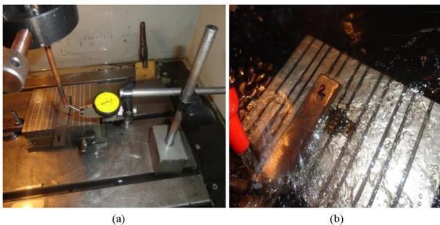
**Fig. 4** Pictorial view of experimental procedure for setting tool electrode and work specimen, (a) application of dial gauge to ensure perfect positioning of tool and specimen, and (b) during machining of specimen
