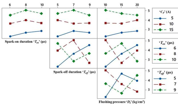
Fig. 10 Influence of variable EDM parameters on average surface roughness for machining DCI using solid cylindrical copper tool electrode
