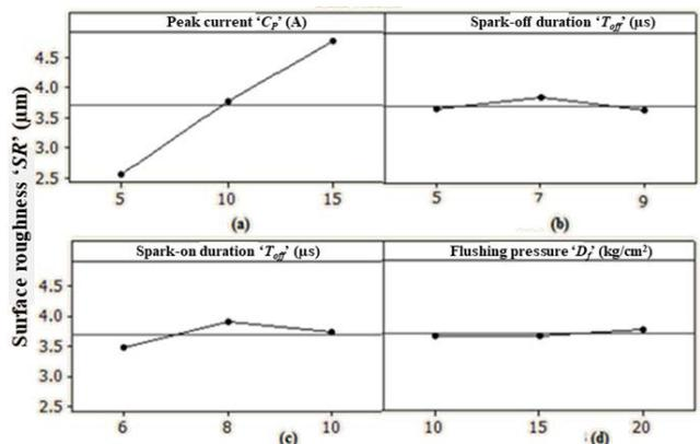
Fig. 9 Influence of variable EDM parameters on average surface roughness for machining DCI using hollow cylindrical copper tool electrode
