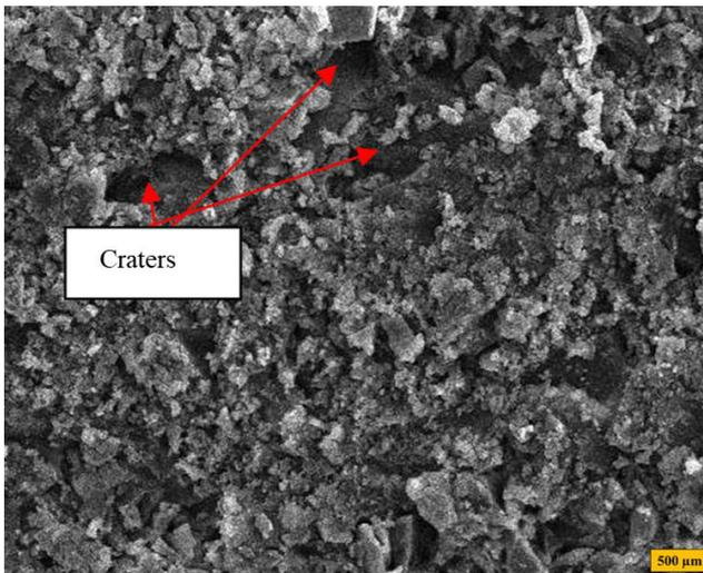
**Fig. 13** Microstructure of eroded surface of DCI machined by EDM using hollow copper electrode
