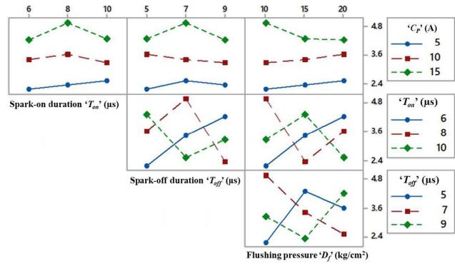
Fig. 11 Interaction among EDM variable parameters for machining DCI using hollow cylindrical copper tool electrode
