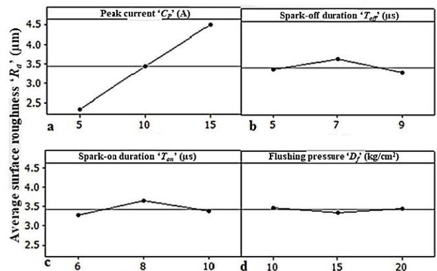
Fig. 8 Influence of variable EDM parameters on average surface roughness for machining DCI using solid cylindrical copper tool electrode
