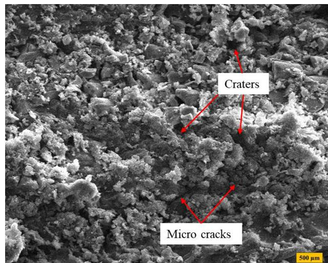
Fig. 12 Microstructure of eroded surface of DCI machined by EDM using solid cylindrical copper electrode
