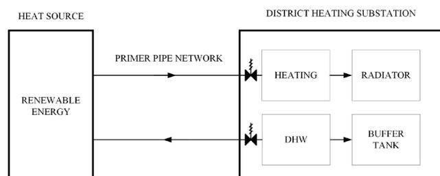
Fig. 1 Conceptual structure of a district heating system
