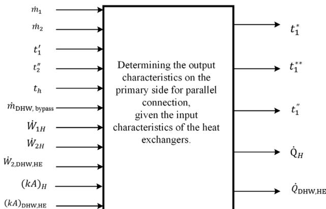
Fig. 6 Relationship between the input and output characteristics for parallel connection
