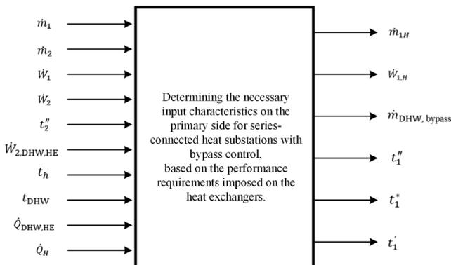
Fig. 7 Relationship of input and output characteristics in a series connection with bypass operation mode
