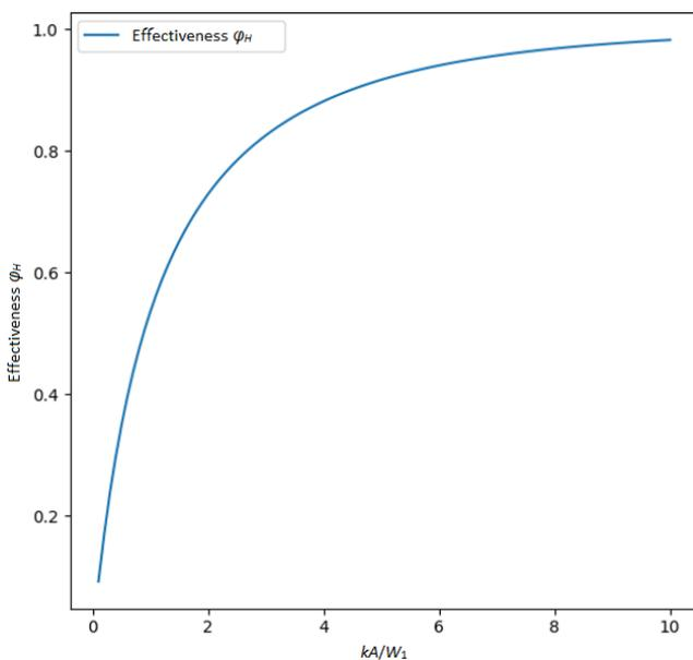
Fig. 9 Effect of the  $kA/W_1$  ratio on heat exchanger efficiency of the heat exchangers
