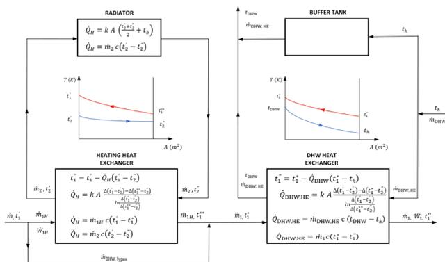
Fig. 4 White box model of a two heat exchanger heat substation on the primary side with serial connection in forward flow mode
