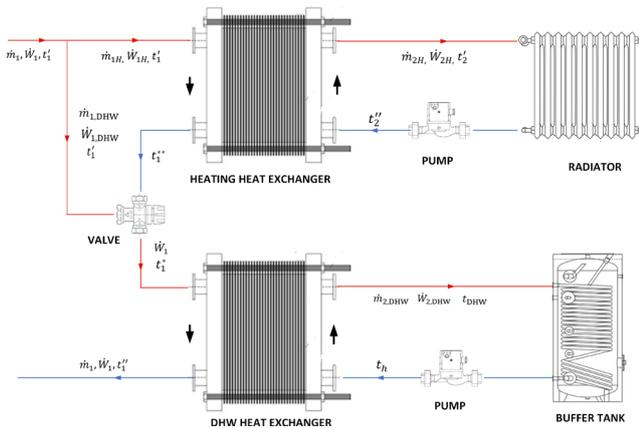
Fig. 2 Block diagram of a heat substation with sequentially connected heating and DHW heat exchangers on the primary side
