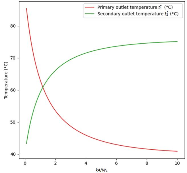
Fig. 10 Effect of the  $kA/W_1$  ratio on the outlet temperatures of the heat exchangers
