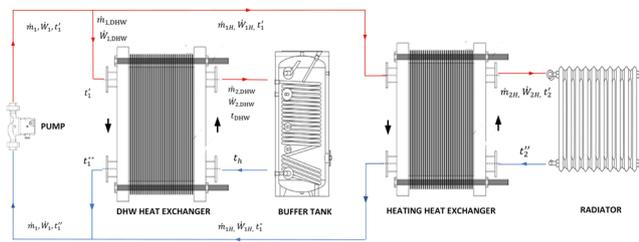
Fig. 3 Block diagram of a heat substation with parallel connections on the primary side
