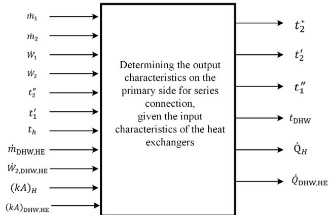
Fig. 5 Relationship between the input and output characteristics on the primary side in a serial connection for the fundamental task
