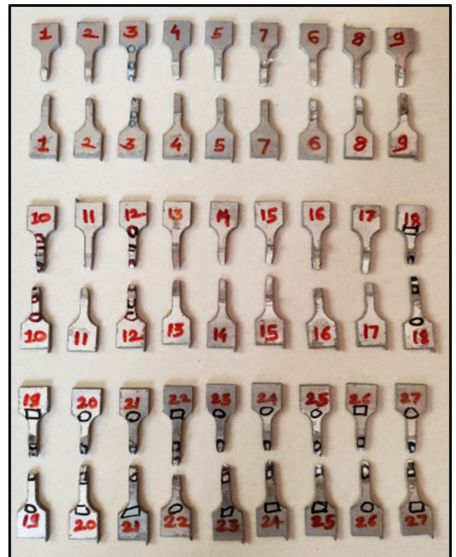
Fig. 5 Water-jet cut tensile specimens prepared from friction stir welded AA3103 plates for mechanical testing
