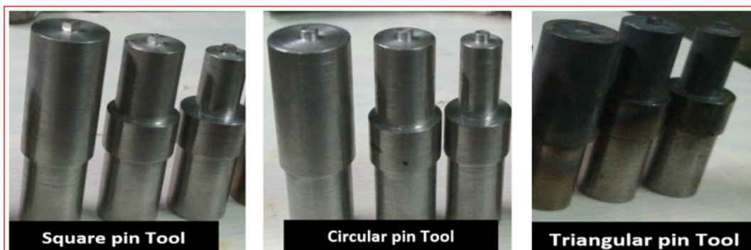
Fig. 2 Tools with different pin profiles – square, circular, and triangular
