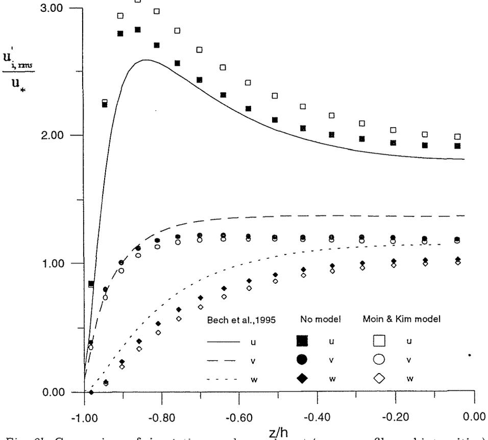
Fig. 3b Comparison of simulations and experiment (mean profile and intensities)
