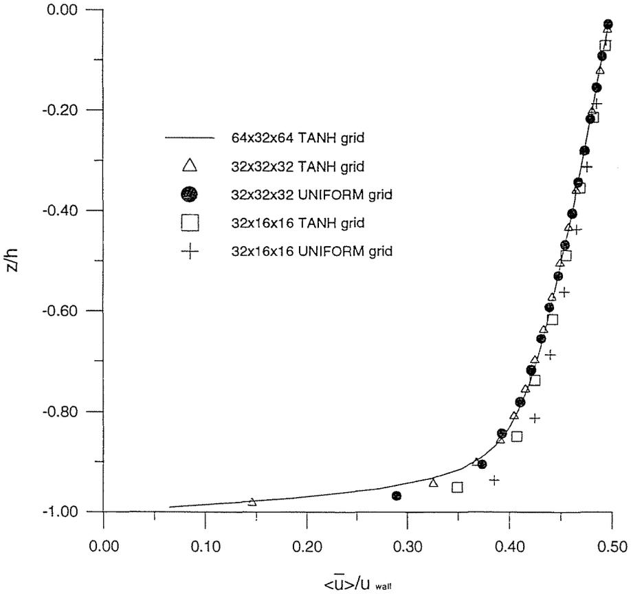
*Fig. 2b* The effect of grid resolution on the mean velocity profile
