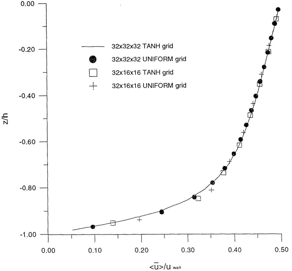
*Fig. 2a* The effect of grid resolution on the mean velocity profile
