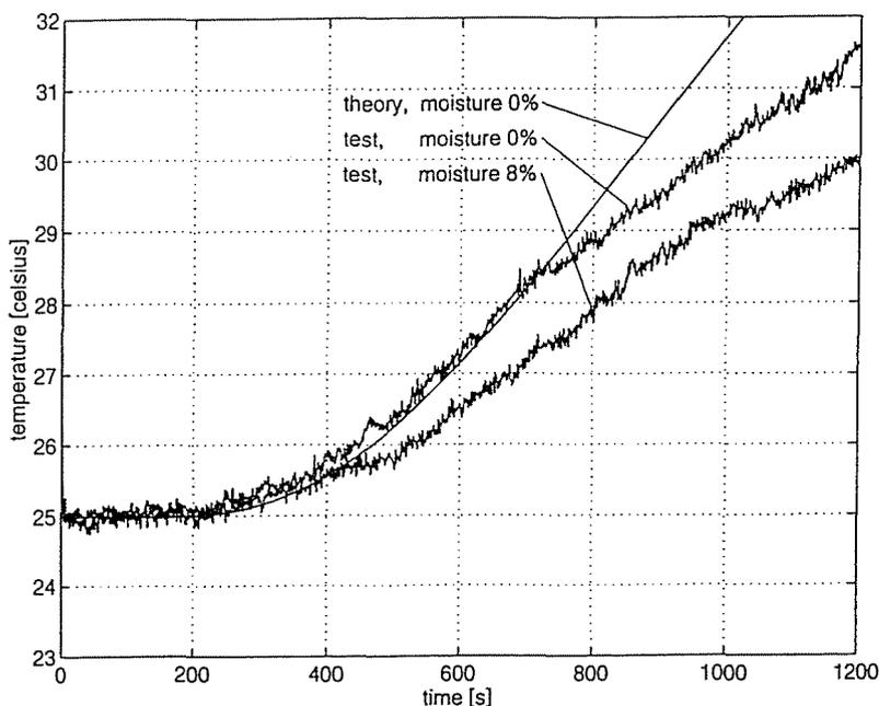
Fig. 4. Temperature vs. time at position 30 mm from the heated end
