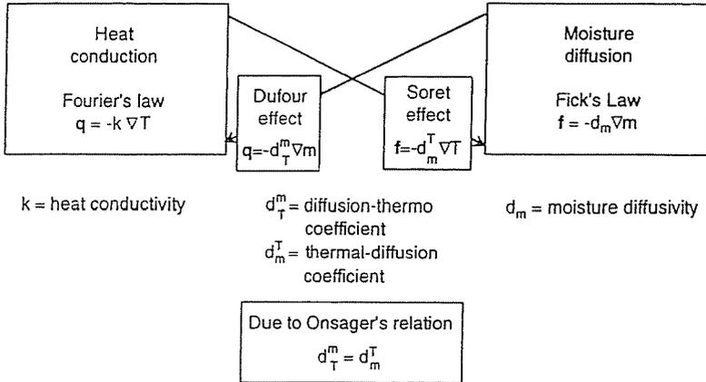
Fig. 1. Coupling of heat conduction and moisture diffusion
