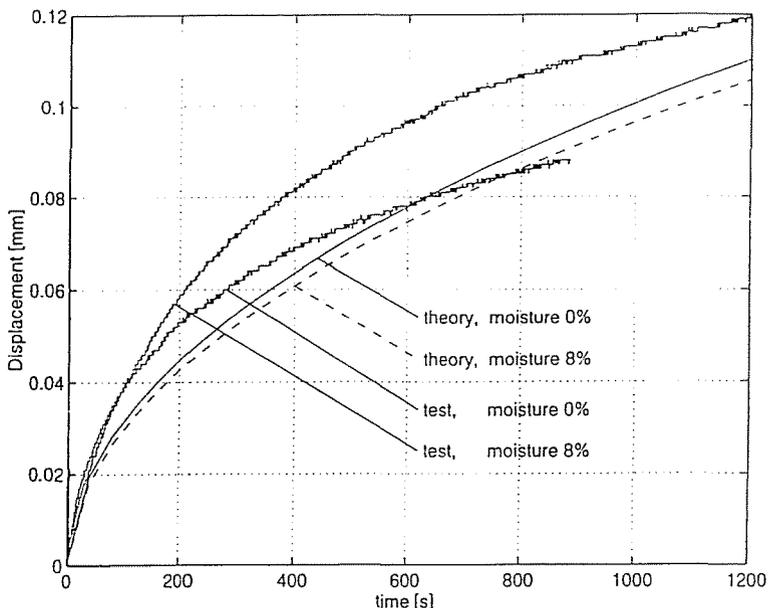
Fig. 5. Displacement vs. time at the free end of test specimen
