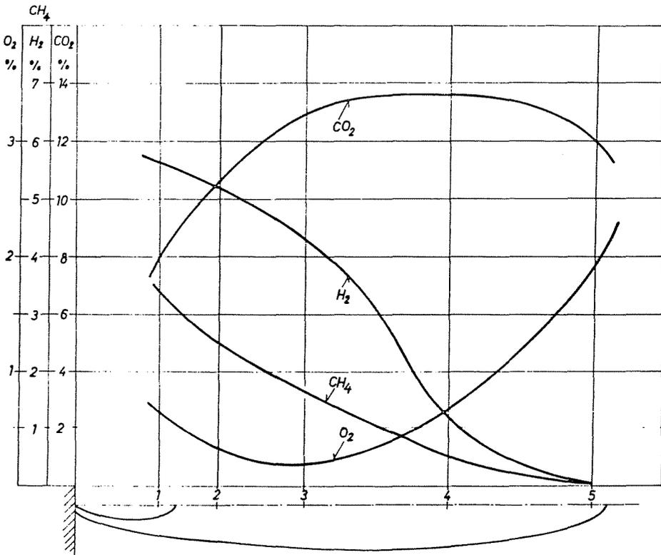
Fig. 2. O<sub>2</sub>, CH<sub>4</sub>, H<sub>2</sub> and CO<sub>2</sub> concentration in the flame (analysed by gas-chromatography)
