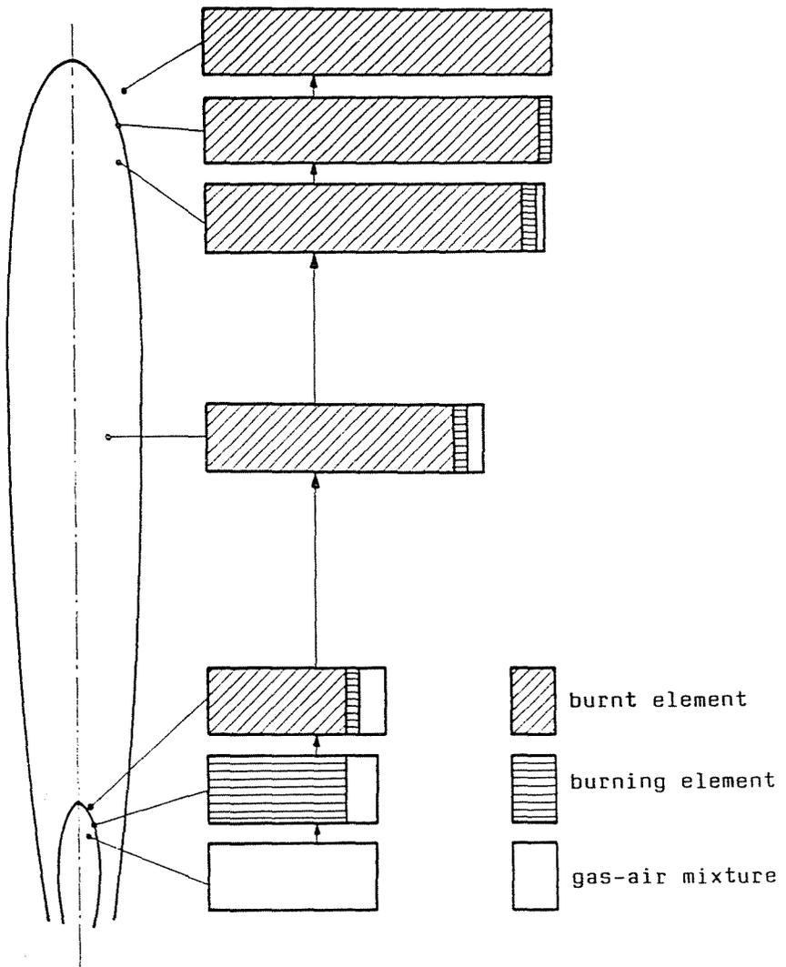
Fig. 6. Different elements in the flame
