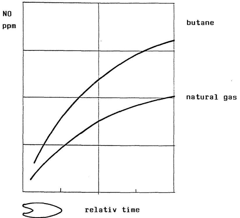
Fig. 8. Calculated NO emission by natural gas and LP
