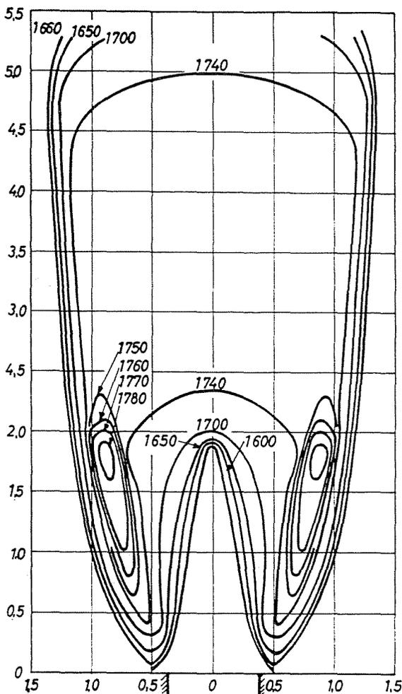
*Fig. 5.* Temperature distribution for a rich flame
