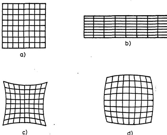
Fig. 4. Examples of raster geometric distortions
