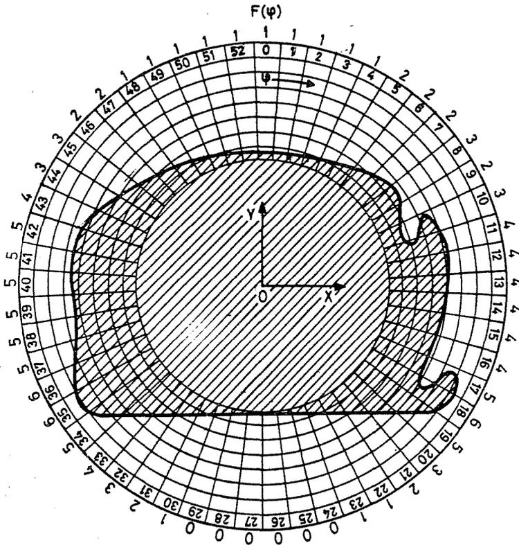
Fig. 3. Projection of image function onto 53-sided regular polygon
