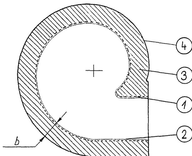
Fig. 4. 1. perforated sheet metal (1.5 mm thick), the hole diameters are 6 mm, the open area ratio is  $\sigma=0.475$
