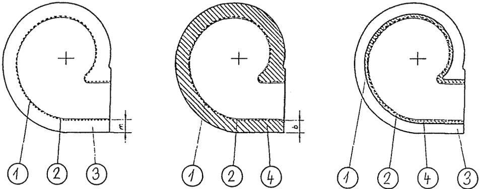
Fig. 9. 1. fabric cover 2. perforated sheet metal 3. cavity 4. sound absorbing material
