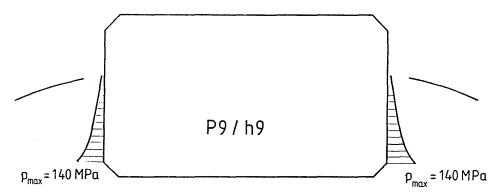
Fig. 10. The pressure distribution due to the interference fit
