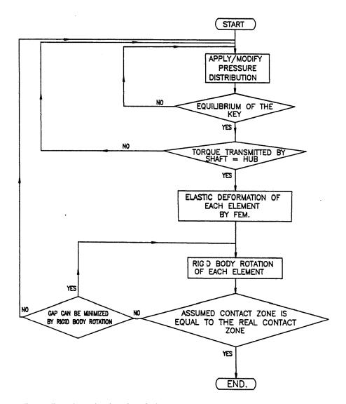
Fig. 4. Flowchart showing the solution process for pressure distribution
