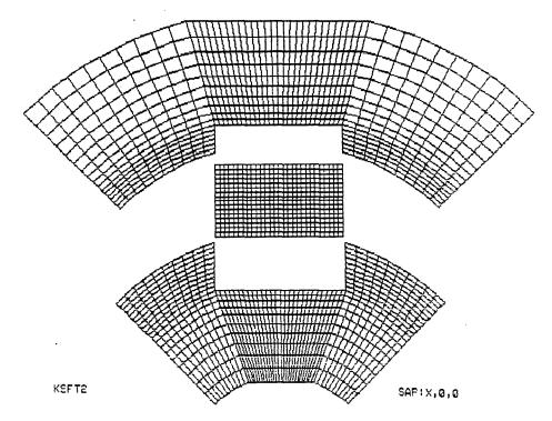
Fig. 5. Finite element mesh of the hub, key and the shaft
