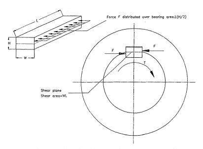
Fig. 1. Idealised force distribution during torque transmission
