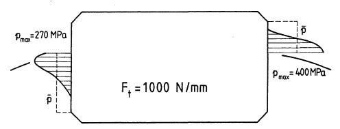
Fig. 7. Pressure distribution on the key (p is the average pressure)
