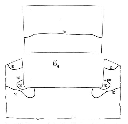
Fig. 12. Von Mises stresses in the shaft and key due to the interference fit
