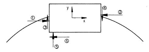
Fig. 2. Resultant forces acting on the key
