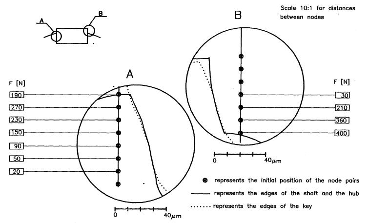
Fig. 6. Figure showing the final positions of the three elements and the magnitude of the normal forces
