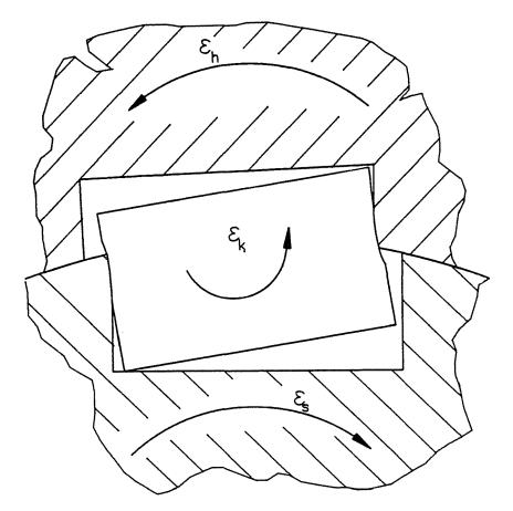
Fig. 3. The deformed elements with rigid body rotation. (The rotations and elastic deformations are enlarged)
