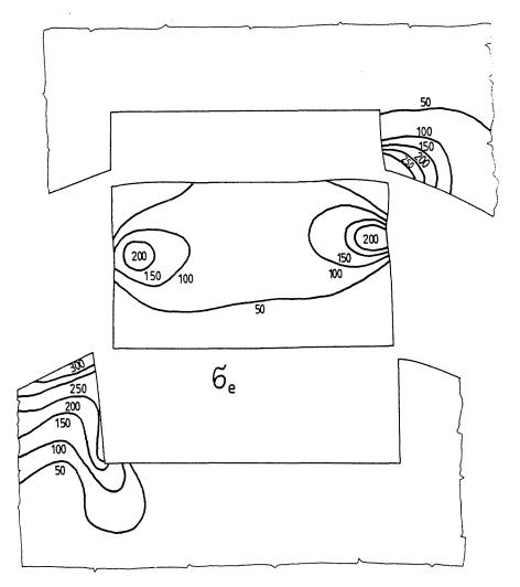
Fig. 9. Von Mises stresses in the shaft, key and hub due to torque transmission
