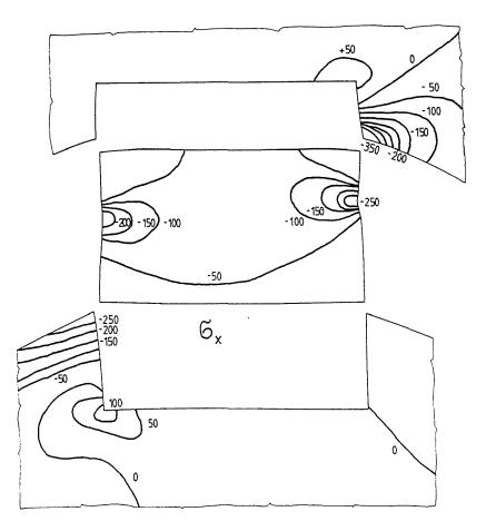
Fig. 8. Horizontal stresses in the shaft, key and hub due to torque transmission
