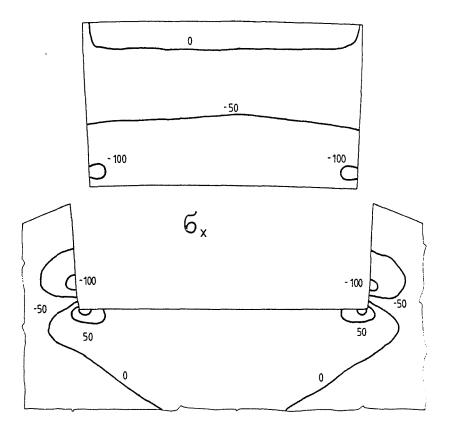
Fig. 11. Horizontal stresses in the shaft and key due to the interference fit
