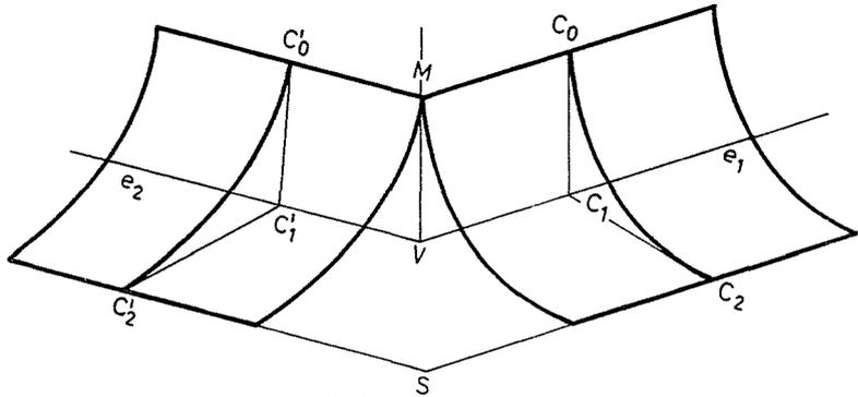
Fig. 2. Neighbouring cylindrical surfaces at a concave vertex
