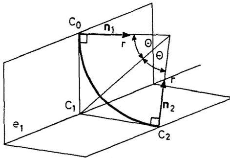
Fig. 1. Conic section defining the cylindrical surface for one edge
