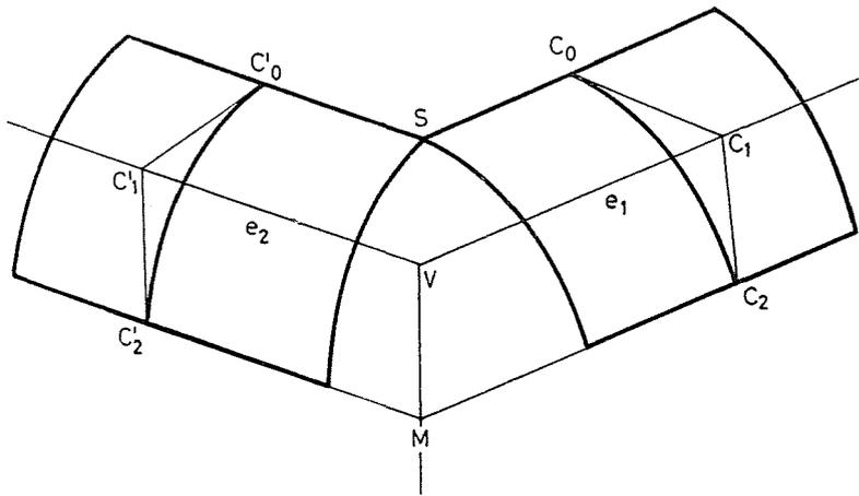
Fig. 3. Neighbouring cylindrical surfaces at a convex vertex
