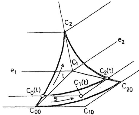
Fig. 7. Triangular patch at concave vertex
