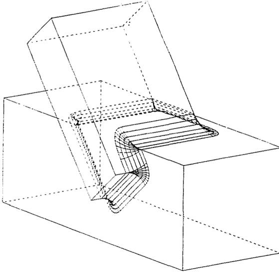
Fig. 9. Blend surface along a closed edge chain
