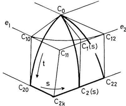
Fig. 8. Four sided patch at convex vertex
