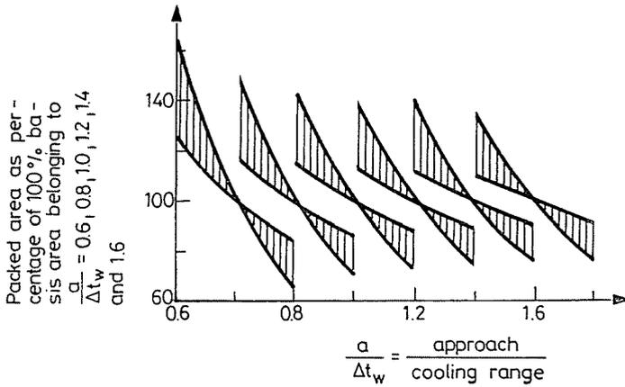
Fig. 3. Variation of cooling tower area as functions of 100 % basic areas belonging to different approach/cooling range values. (Characteristic data of the tested region:  $p_{bar} = 1.0$  bar;  $5.0 \leq t_{wb} \leq 30$  °C;  $3.0 \leq \Delta t_w \leq 21.0$  °C;  $1.2 \leq C \leq 3.0$ ;  $0.5 \leq m \leq 0.9$ ).
