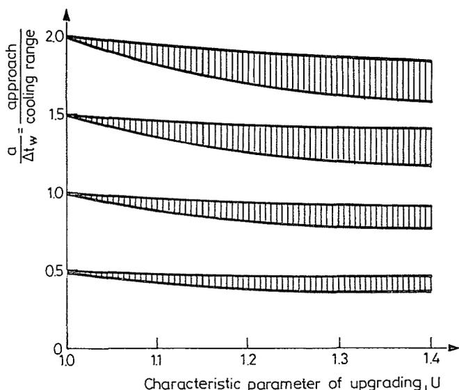
Fig. 6. Approach/cooling range variation as a function of  $U$  at constant fan power before and after upgrading (Characteristic data of the tested region:  $p_{\text{bar}} = 1.0$  bar,  $5.0 \leq t_{wb} \leq 30$  °C;  $3.0 \leq \Delta t_w \leq 21.0$  °C;  $1.2 \leq C \leq 3.0$ ;  $0.5 \leq m \leq 0.9$ ).
