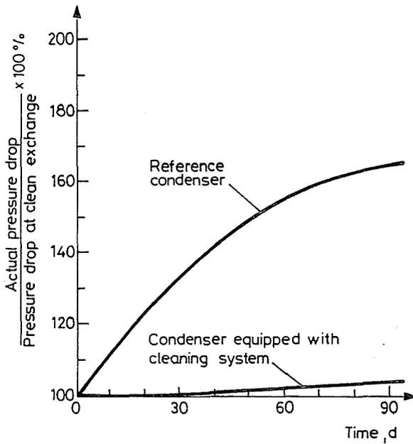
Fig. 9. Heat transfer and pressure loss at a condenser equipped with on-load brush cleaning system and at a reference condenser (measured values).
