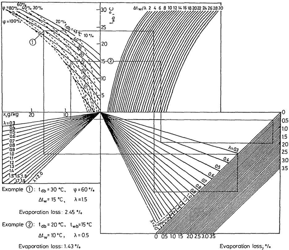
Fig. 10. Generalized chart for the determination of evaporation loss of cooling towers [4]
