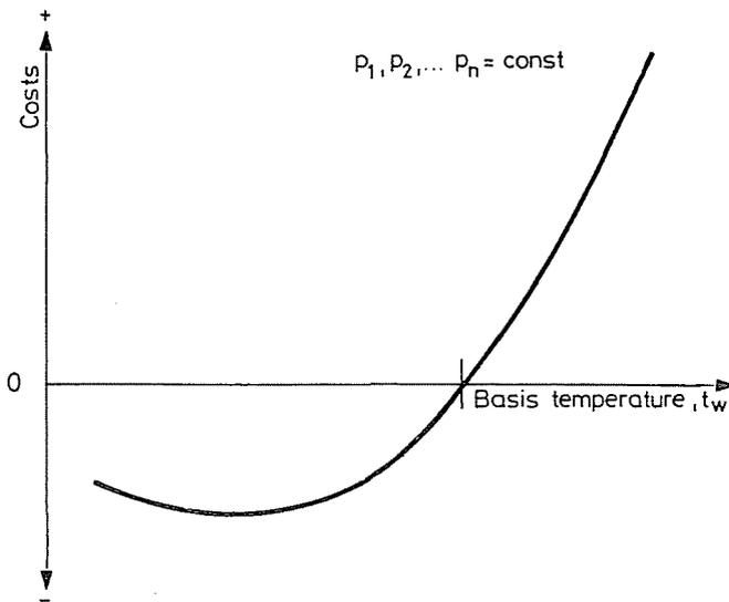
Fig. 7. Costs versus cold water temperature
