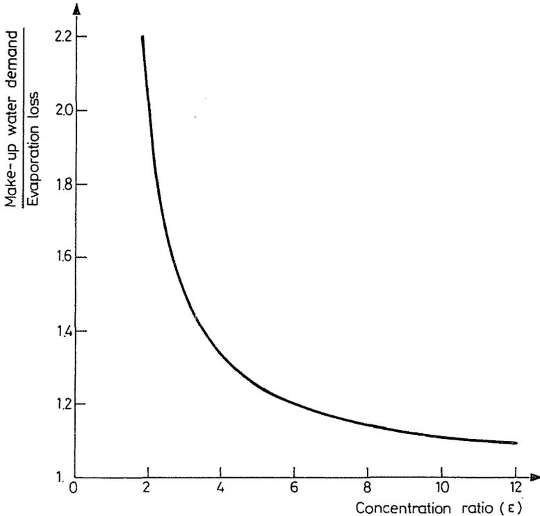
Fig. 12. Ratio of make-up water flow and evaporation loss as a function of concentration ratio
