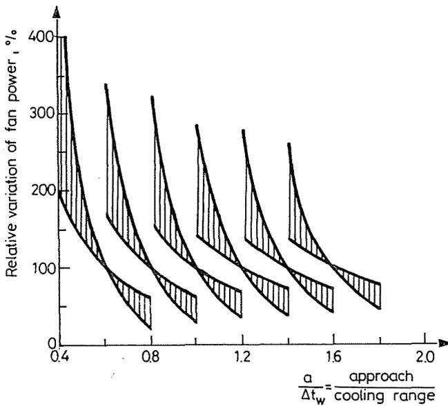
Fig. 4. Correlation of fan power and cooling performance (Characteristic data of the tested region:  $p_{\text{bar}} = 1.0$  bar;  $5.0 \leq t_{wb} \leq 30$  °C;  $3.0 \leq \Delta t_w \leq 21.0$  °C;  $1.2 \leq C \leq 3.0$ ;  $0.5 \leq m \leq 0.9$ ).
