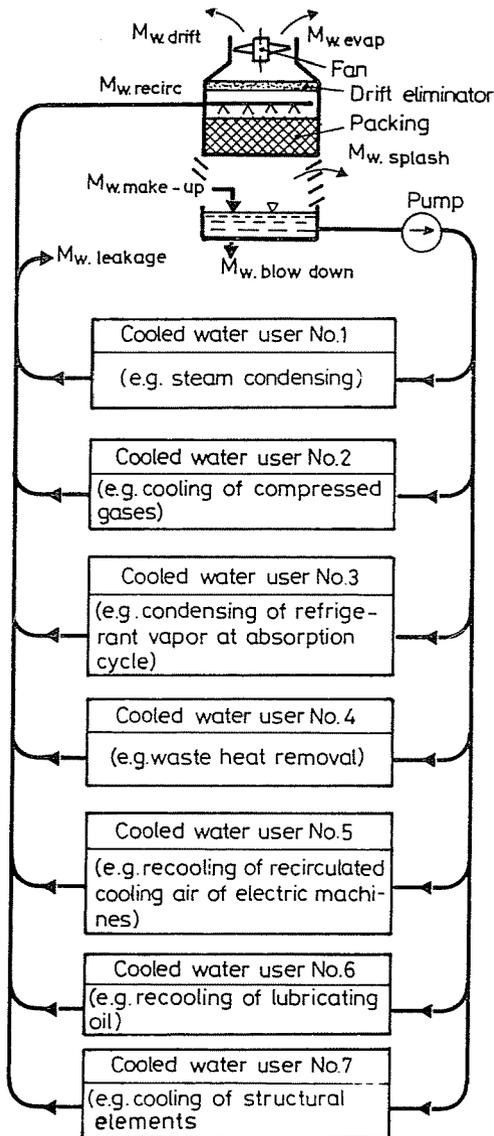
Fig. 1. Scheme of a cooling cycle with mechanical draft cooling tower supplying cold water for different users
