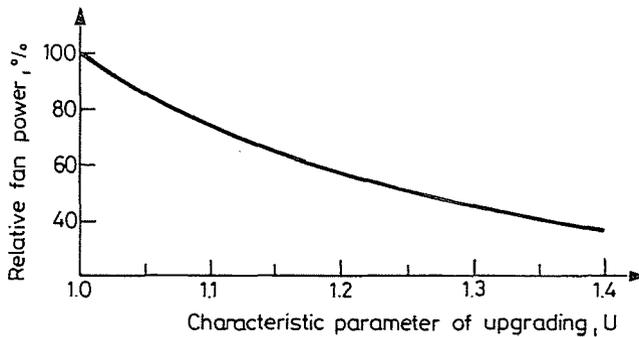
Fig. 5. Fan power variation with characteristic parameter of upgrading,  $U$ . (Characteristic data of the tested region:  $p_{\text{bar}} = 1.0$  bar;  $5.0 \leq t_{wb} \leq 30$  °C;  $3.0 \leq \Delta t_w \leq 21.0$  °C;  $1.2 \leq C \leq 3.0$ ;  $0.5 \leq m \leq 0.9$ ).
