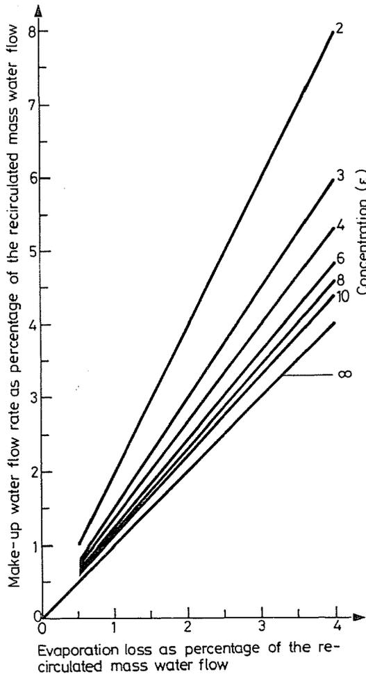
Fig. 11. Make-up water flow as functions of evaporation loss and concentration ratio
