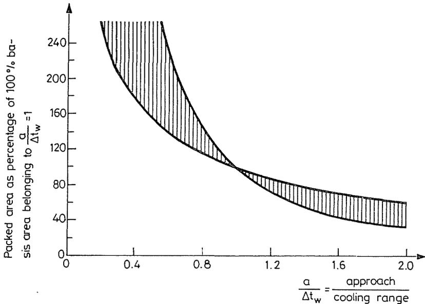
Fig. 2. Variation of cooling tower area as a function of approach/cooling range (Characteristic data of the tested region:  $p_{\text{bar}} = 1.0 \text{ bar}$ ;  $5.0 \leq t_{wb} \leq 30 \text{ }^\circ\text{C}$ ;  $3.0 \leq \Delta t_w \leq 21.0 \text{ }^\circ\text{C}$ ;  $1.2 \leq C \leq 3.0$ ;  $0.5 \leq m \leq 0.9$ ).
