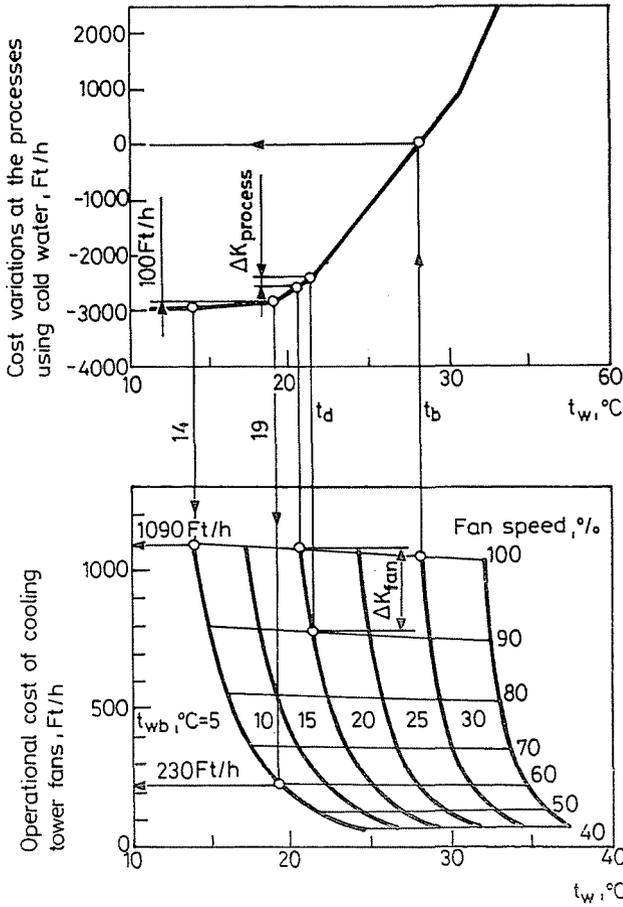
Fig. 8. Determination of distinct cold water temperature  $t_d$  ( $\Delta K_{process} = \Delta K_{fan}$ )
