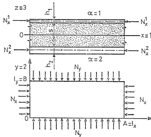
Fig. 2. The loading of the sandwich plate
