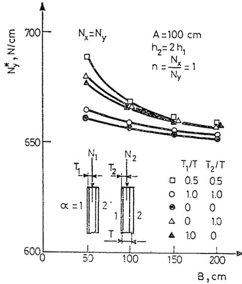
Fig. 6. Effect of the variation of the planes of external forces for the critical loads
