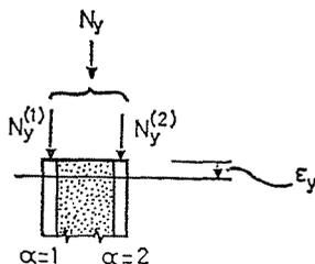
Fig. 4. Deformation in bending-less state
