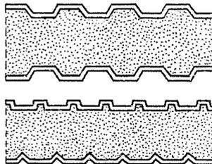
Fig. 1. The construction of the sandwich plate
