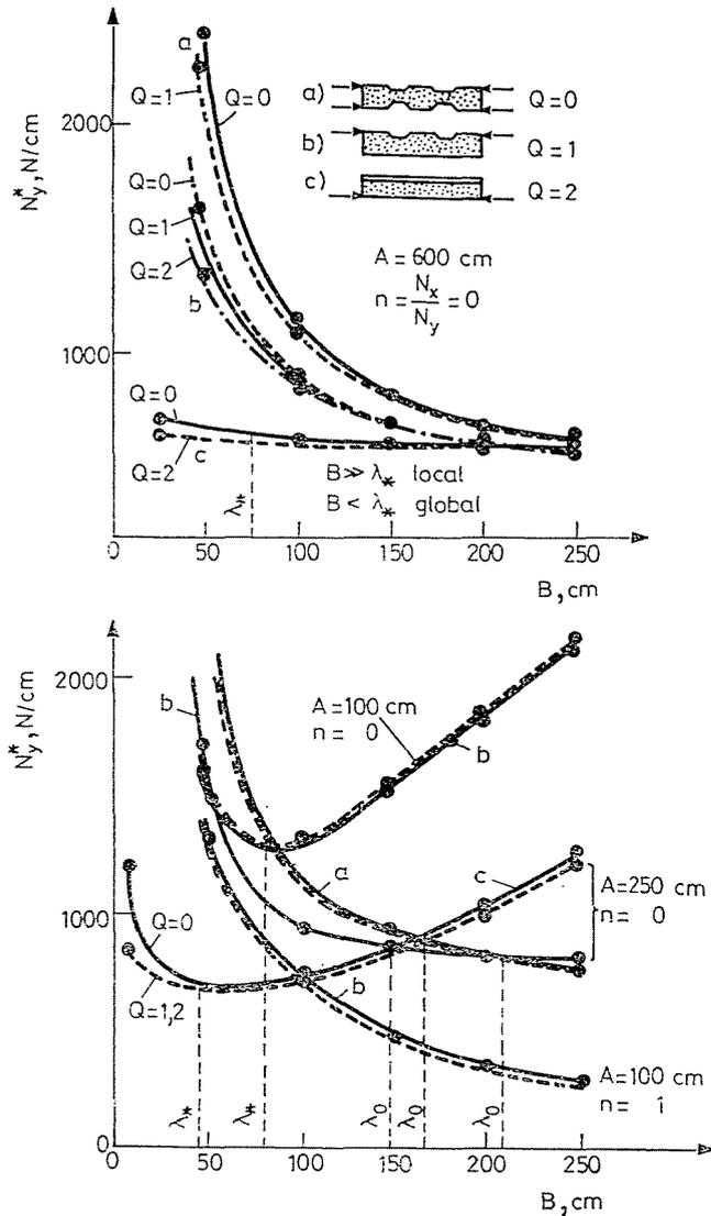
Fig. 5. Critical loads vs. side length  $B$  for different case of construction (a, b, c) loading ( $Q=0, 1, 2$ ) and side length  $A$
