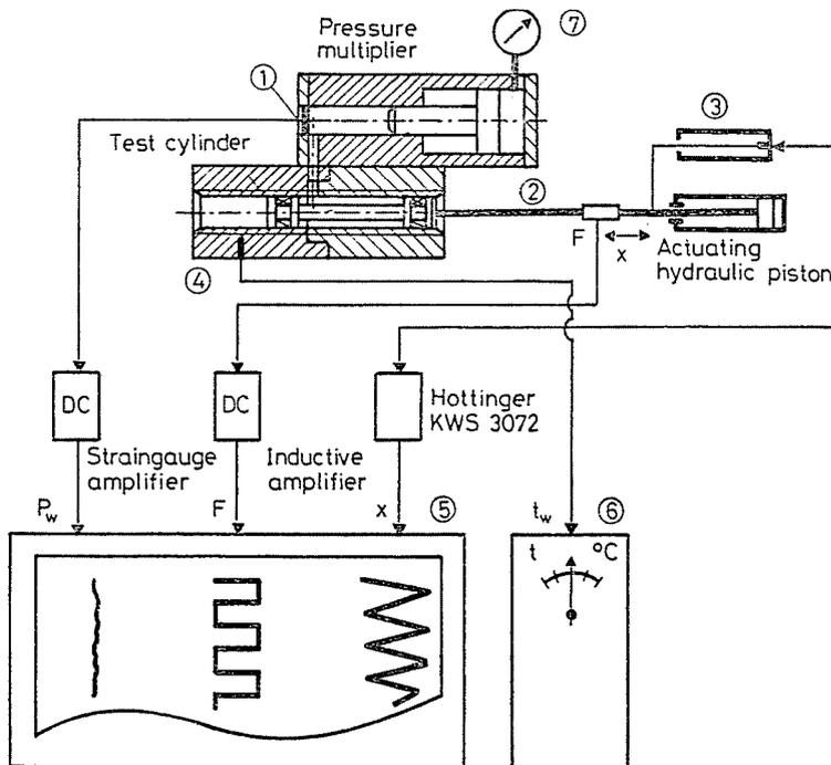
Fig. 3. Measuring system of the test rig
