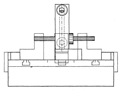
Fig. 5. Front-view design of a workpiece clamping fixture
