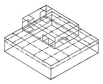
Fig. 3. Envelope surface of a workpiece with zones, and pallet (base plate) in the Jig & Fix CAD system
