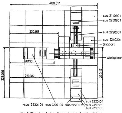
Fig. 6. Top-view design of a workpiece clamping fixture
