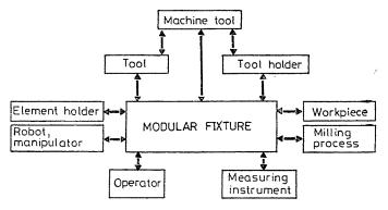
Fig. 2. Factors affecting the construction of the fixtures
