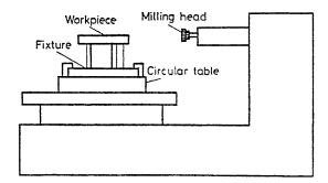
Fig. 1. Connection between workpiece, clamping fixture and milling machine
