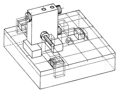
Fig. 7. Display of a workpiece clamping fixture from an arbitrary viewpoint
