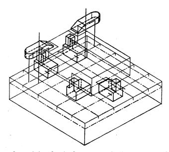
Fig. 4. A complete workpiece clamping fixture surrounding the workpiece envelope surface
