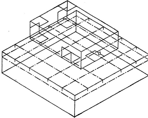
Fig. 3. Envelope surface of a workpiece with zones, and pallet (base plate) in the Jig & Fix CAD system
