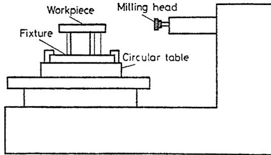
Fig. 1. Connection between workpiece, clamping fixture and milling machine
