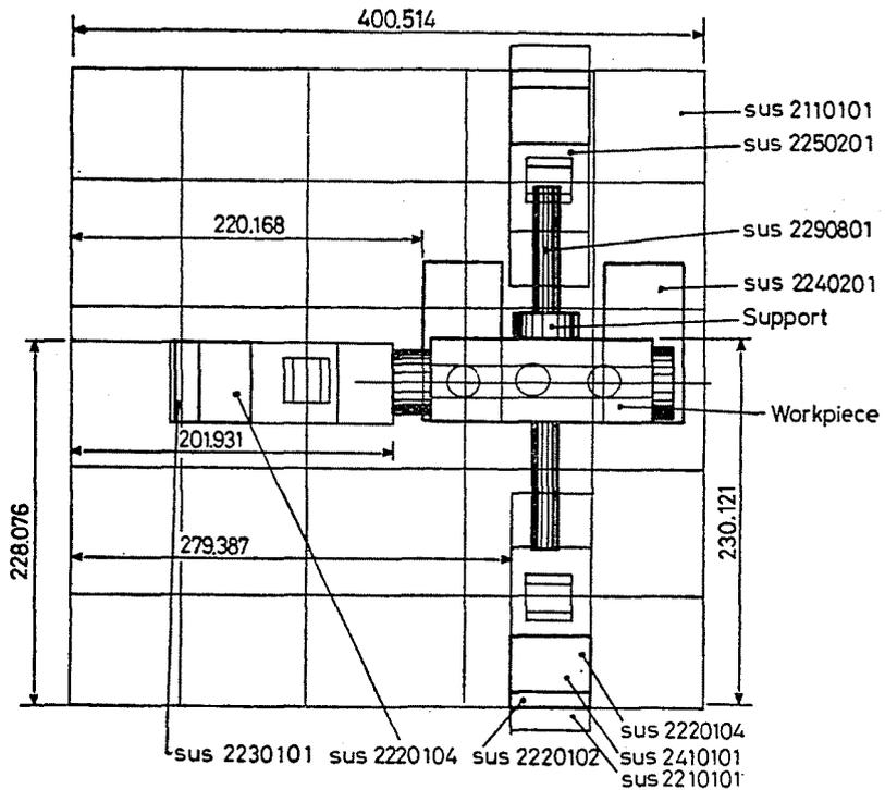
Fig. 6. Top-view design of a workpiece clamping fixture
