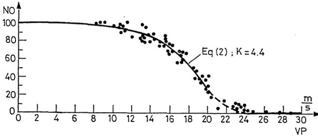
Fig. 5. The relation between the particle velocity and the number of unbroken particles (ALO:  $dr=5-5.3$  mm;  $\alpha=90^\circ$ )
