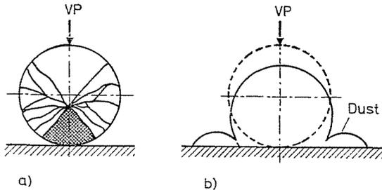
Fig. 3. The degradation of a single particle: a) Zones of degradation at impact; b) a particle in the process of impacting on a hard surface. (From Uuemois, Ref 6.)
