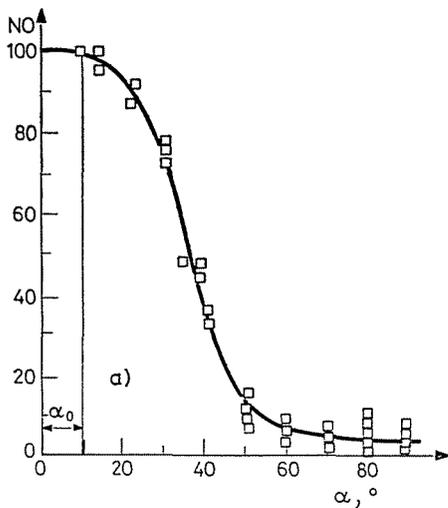
Fig. 10a. The effect of the impact angle on the number of unbroken particles (AIO particles:  $d_r=5-5.3$  mm: steel target 5 mm thickness:  $VP=23$  m/sec)
