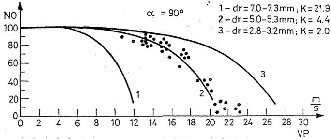
Fig. 14. The relation between the particle velocity and the number of unbroken particles for different particle diameters (AIO)
