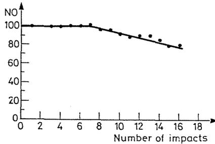
Fig. 13. The relation between the number of impacts and the number of unbroken particles (POL:  $dr = 7.4-7.6 \text{ mm}$ )
