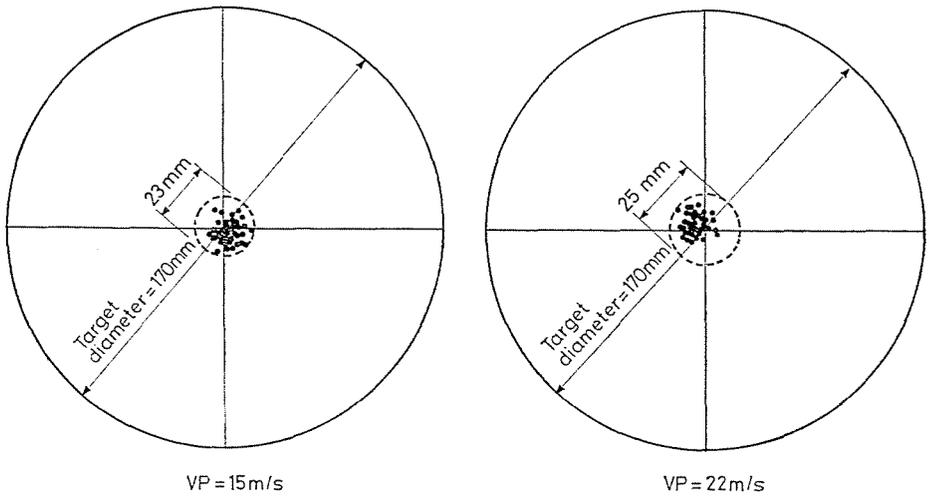
Fig. 20. The position of impact of 100 particles (AIO:  $dr=5-5.3$  mm:  $\alpha=90^\circ$ ) on a steel target (5 mm thickness) in the case of  $VP=15$  m/sec and the case of  $VP=22$  m/sec
