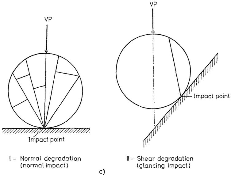
Fig. 10c. The two types of degradation
