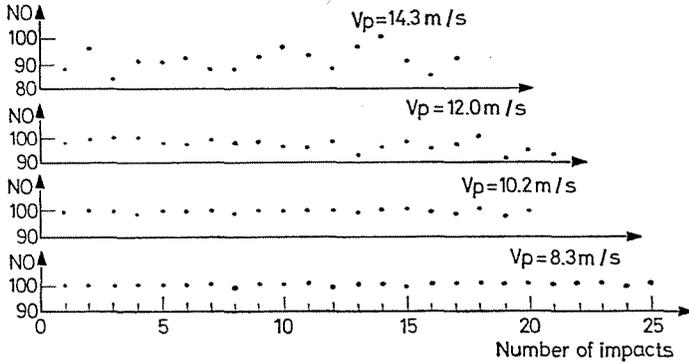
Fig. 12. The effect of the number of impacts on the number of unbroken particles at different particle velocities (AIO:  $dr = 5-5.3 \text{ mm}$ ;  $\alpha = 90^\circ$ )
