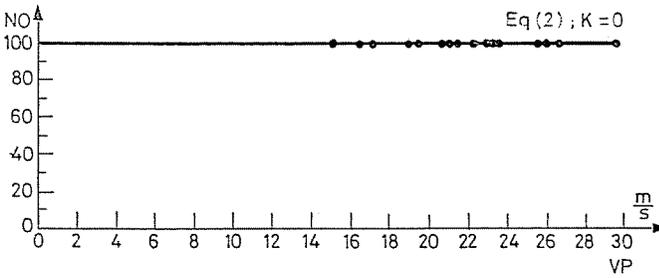
Fig. 8. The relation between the particle velocity and the number of unbroken particles (GLS:  $dr=5$  mm;  $\alpha=90^\circ$ )
