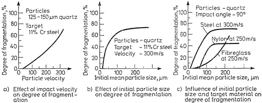
Fig. 2. a) Effect of impact velocity on degree of fragmentation; b) Effect of initial particle size on degree of fragmentation; c) Influence of initial particle size and target material on degree of fragmentation
