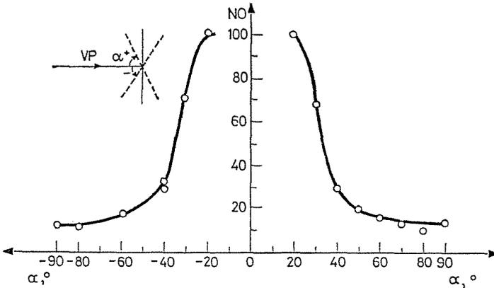
Fig. 18. The effect of the sign of the impact angle on the number of unbroken particles (AIO)  $dr = 4.6-5.4$  mm:  $VP = 22$  m/sec
