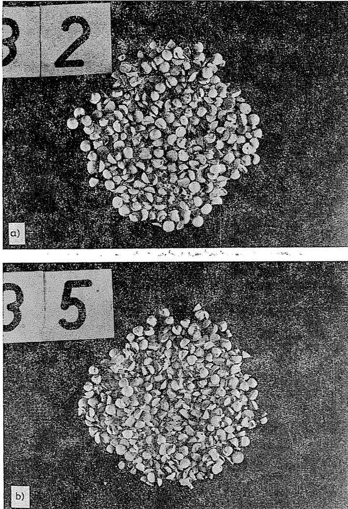
*Fig. 6.* The effect of increasing the velocity on the size of the broken particles (AIO:  $dr=5-5.3$  mm)
