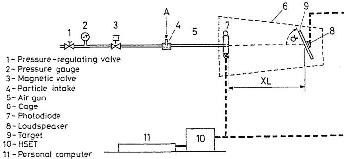
Fig. 4. Schema of impact test apparatus and arrangement of measuring systems
