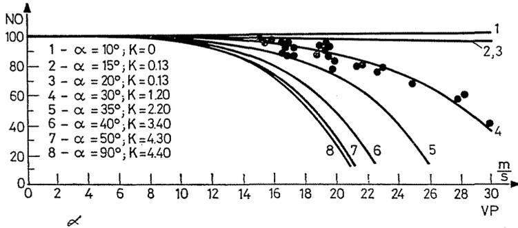
Fig. 9. The relation between the particle velocity and the number of unbroken particles for different impact angles (ALO:  $dr=5-5.3$  mm)
