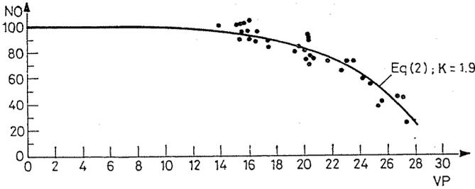
Fig. 7. The relation between the particle velocity and the number of unbroken particles (POL:  $dr=7.4-7.6$  mm;  $\alpha=90^\circ$ )
