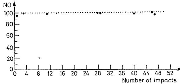
Fig. 11. The relation between the number of impacts and the number of unbroken particles (AlO:  $dr=4.9-5$  mm:  $VP=9.3$  m/sec:  $\alpha=90^\circ$ )
