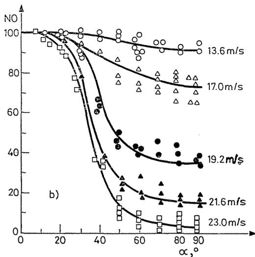
Fig. 10b. The effect of the angle on the number of unbroken particles in the case of constant particle velocity (For AIO particles:  $d_r=5-5.3$  mm: steel target of 5 mm thickness)
