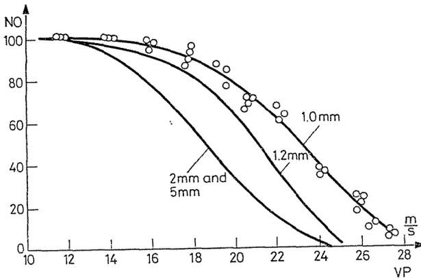
Fig. 15. The effect of the target thickness (steel) on the number of unbroken particles (AIO particles:  $dr=5-5.3$  mm: steel target: impact angle  $=90^\circ$ )
