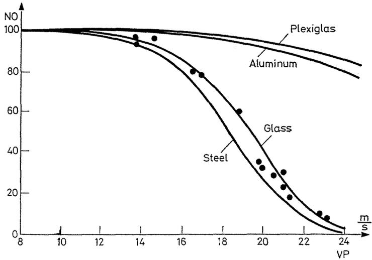
Fig. 17. The effect of the type of the target material on the number of unbroken particles (AIO particle:  $d_r = 5-5.3$  mm: target thickness = 5 mm: impact angle =  $90^\circ$ )
