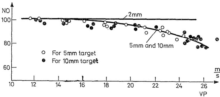
Fig. 16. The effect of the target thickness (plexiglas) on the number of unbroken particles (AIO particles:  $dr=5-5.3$  mm: plexiglas target: impact angle  $=90^\circ$ )
