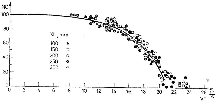
Fig. 19. The relation between the particle velocity and the number of unbroken particles for different  $XL$  values (AIO:  $dr = 5-5.3$  mm:  $\alpha = 90^\circ$ )
