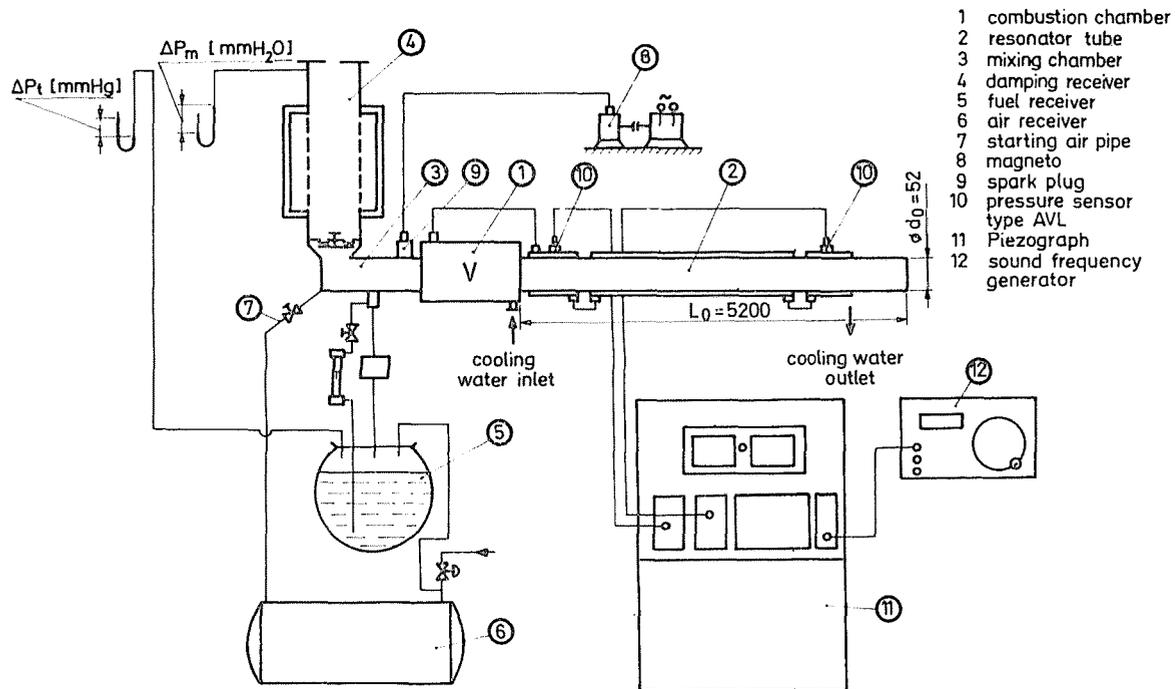
Fig. 3. Scheme of experimental equipment — layout and instrumentation
