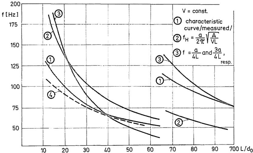
Fig. 4. Influence of resonator tube length on frequency of the oscillating system
