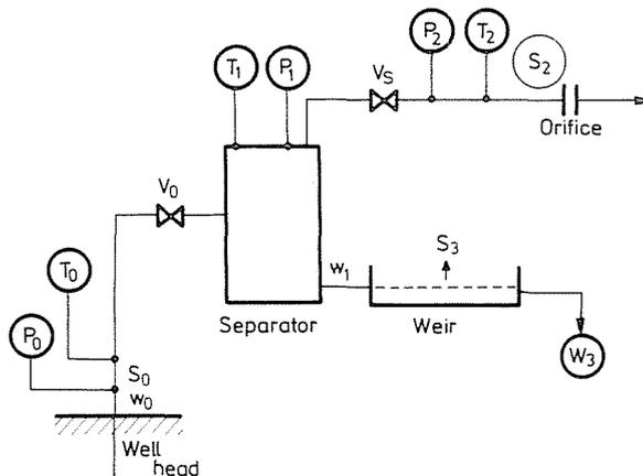
Fig. 5. Systematic diagram of the measurement using the steam—water separator
