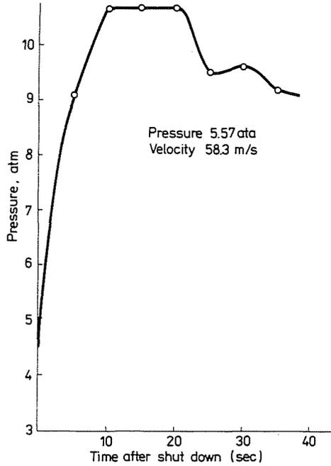
Fig. 25. Pressure fluctuation by sudden shut-down of discharge valve (Max. flow)
