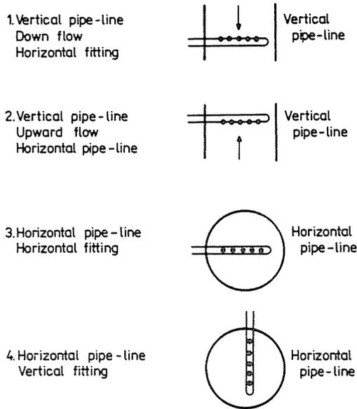
Fig. 8. Desirable order of the sampling nozzle position. 1. Vertical pipe-line. Down flow. Horizontal fitting; 2. Vertical pipe-line. Upward flow. Horizontal pipe-line; 3. Horizontal pipe-line. Horizontal fitting; 4. Horizontal pipe-line. Vertical fitting
