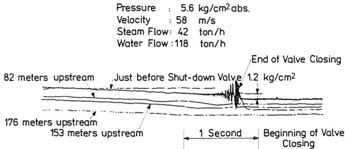
Fig. 26. Oscillograph of pressure change in the transmission pipe-line at sudden shut-down of discharge valve
