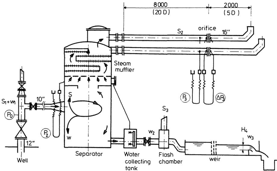
Fig. 21. Improved design of open-type separator combined with steam muffler
