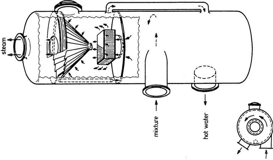
Fig. 16. Pressure type separator (C)
