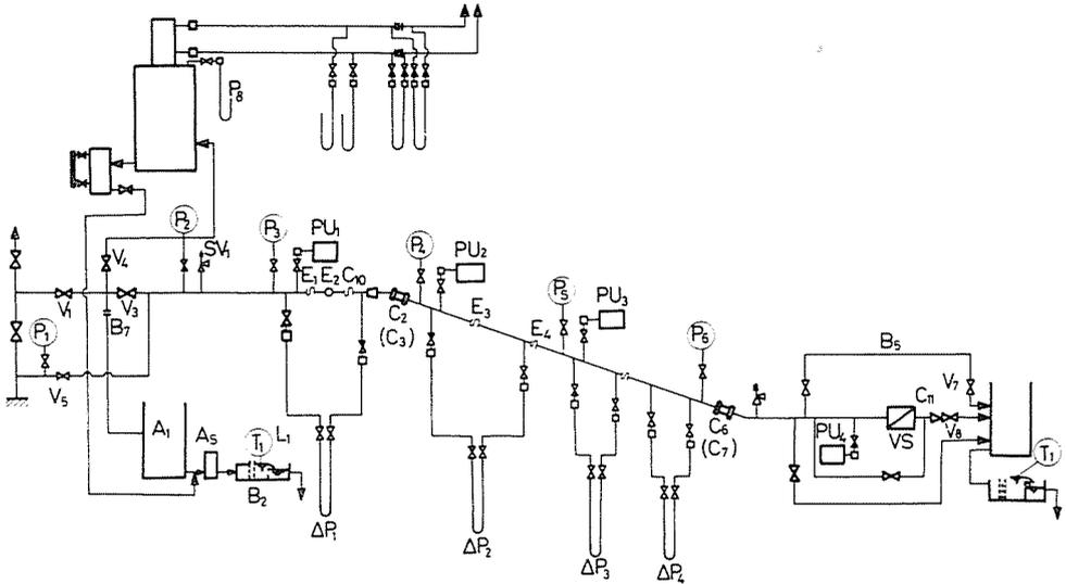
Fig. 24. Systematic diagram of the mixture transmission system on test loop
