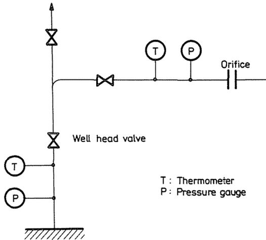
Fig. 2. Measurement of the steam flow rate
