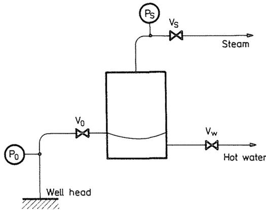
Fig. 3. Measurement using the steam—water separation
