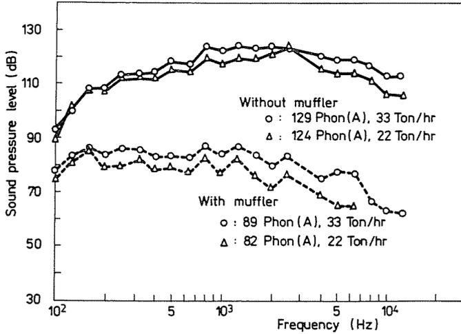
Fig. 19. Sound pressure level with and without muffler
