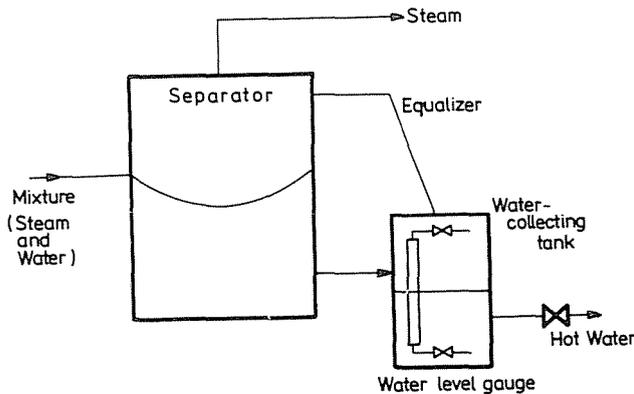
Fig. 11. Steam—water separator equipped with a water collecting tank
