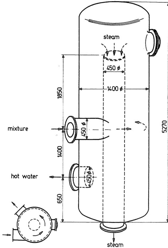
Fig. 14. Pressure type separator (A)
