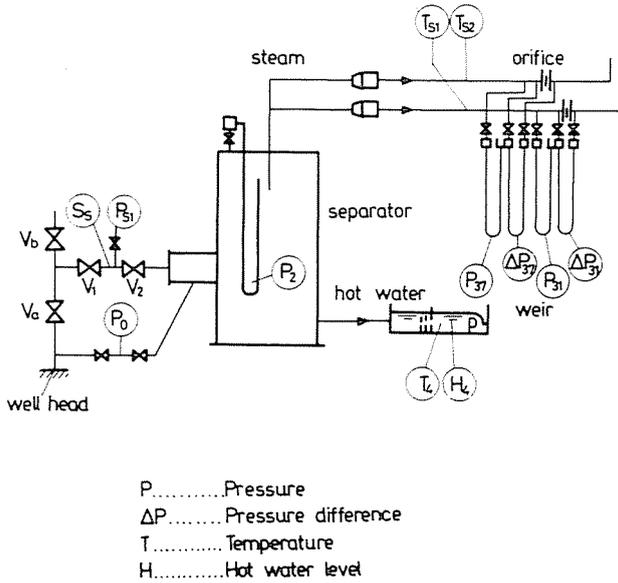
Fig. 12. Systematic diagram of the measurement by open type separator. P ... Pressure;  $\Delta P$  ... Pressure difference; T ... Temperature; H ... Hot-water level
