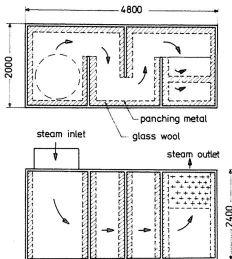
Fig. 18. Construction of steam muffler
