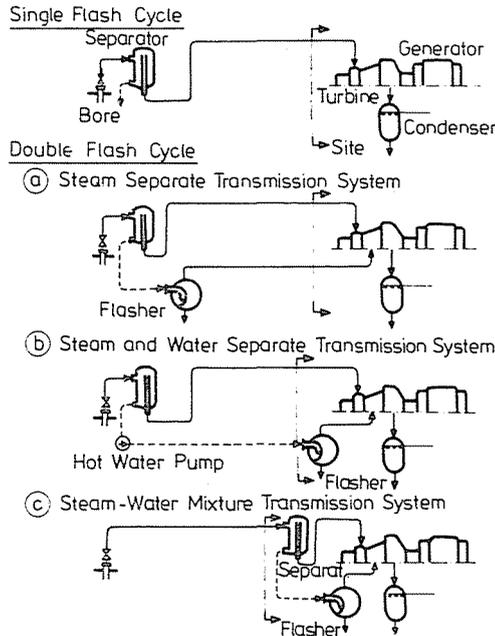
Fig. 22. Hot-water type geothermal power plant cycle and transmission system
