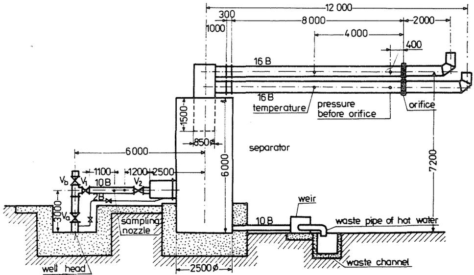
Fig. 13. Open type separator with measuring pipe-line
