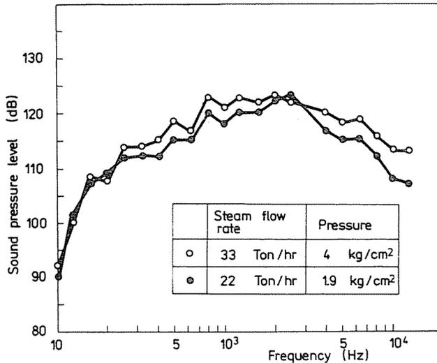
Fig. 17. Frequency spectra of steam flashing noise
