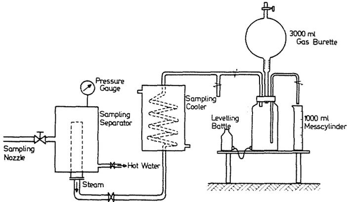
Fig. 10. Apparatus of the measurement of non-condensable gases
