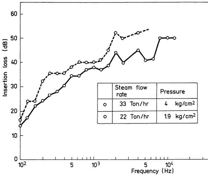
Fig. 20. Noise reduction by steam muffler
