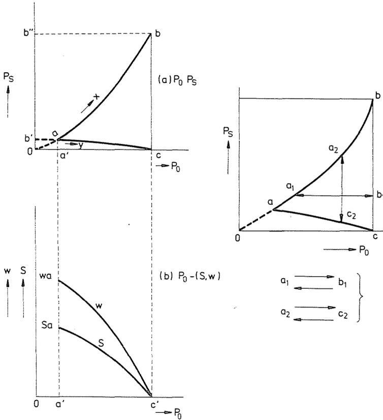
Fig. 4. Relation between well head pressure ( $P_0$ ) and outlet of separator ( $P_s$ ), steam flow rate ( $S$ ), hot water flow rate ( $W$ )
