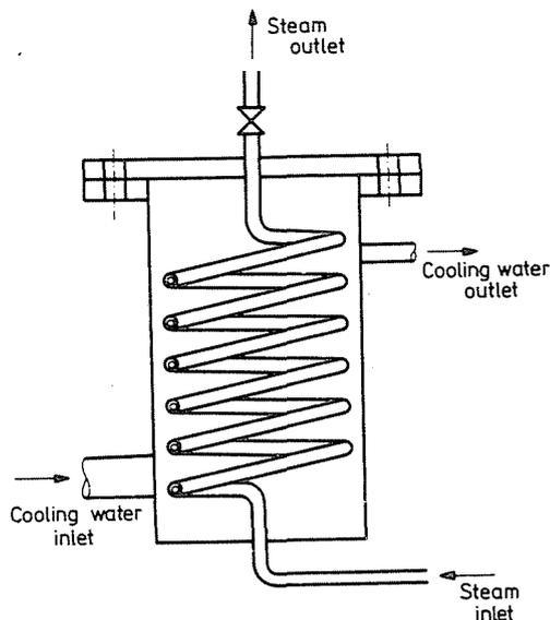
Fig. 9. Cooling equipment of the sampling steam
