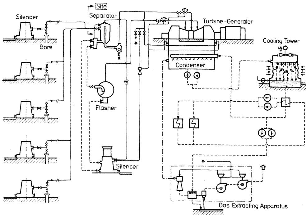
Fig. 23. 50 MW double-flash-cycle plant (Hachobaru Power Station)
