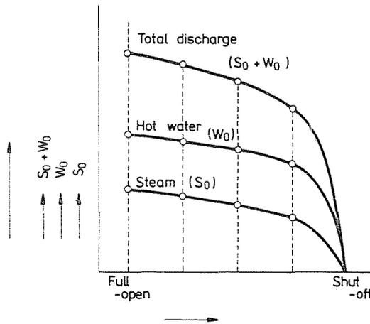
Fig. 6. Physical well characteristics
