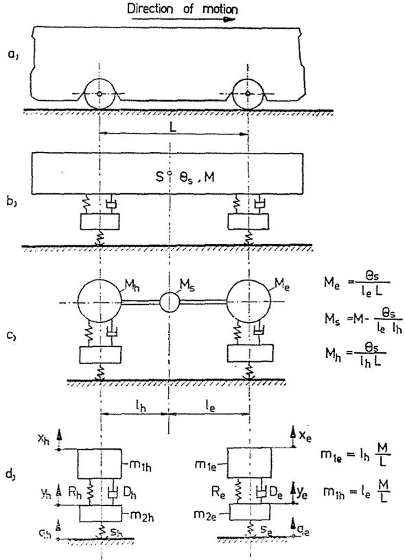
Fig. 3. Deduction of the vibration model for the bus
