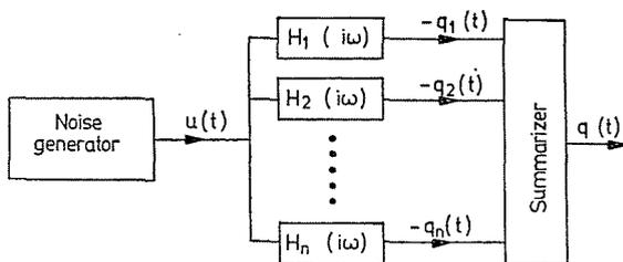
Fig. 1. Principle of modelling random signals
