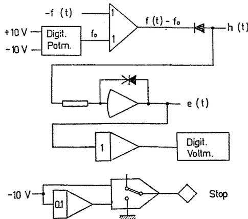
Fig. 6. Program of the statistical processing of the analogue signal
