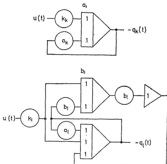
Fig. 2. Filter circuits to be adjusted on the analogue computer
