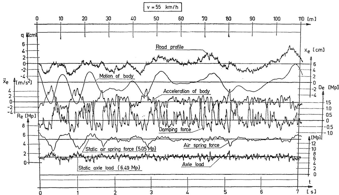
Fig. 5. Motion characteristics for the front part of a loaded bus travelling on a good quality asphalt road
