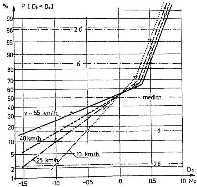
Fig. 9. Distribution functions for damping force, if the loaded bus travels on a good quality asphalt road
