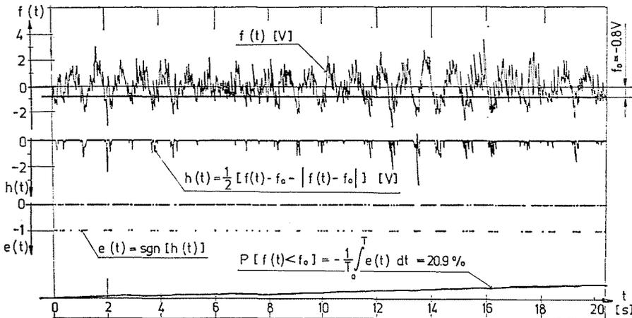
Fig. 7. Formation of signals in the course of statistical processing
