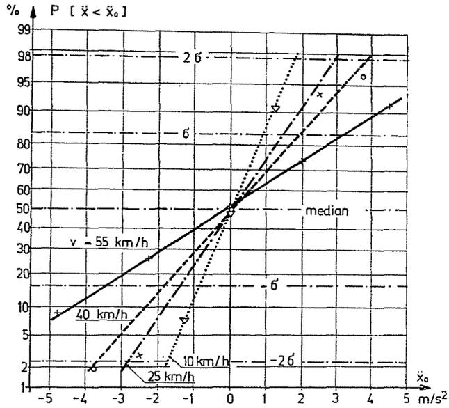
Fig. 8. Distribution functions for accelerations at the front part of a loaded bus traveling on a good quality asphalt road
