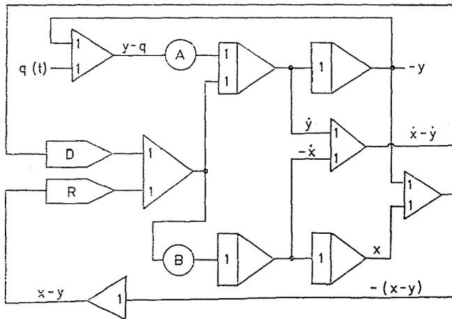
Fig. 4. Analogue program of the vibration system of the bus
