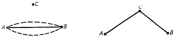
Fig. 8. The effect of vibration on a dislocation fixed in two nodes, in the stress-free state
