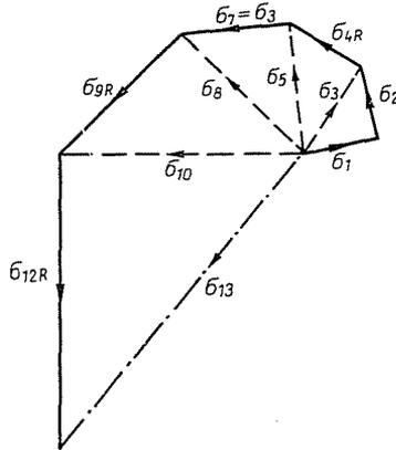
Fig. 8. Construction of error propagation from components, at HRC 30
