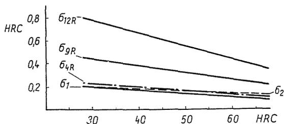
Fig. 4. Standard deviations of error components in Rockwell C measurements, in function of hardness.  $\sigma_1$ , measuring process and apparatus;  $\sigma_2$ , long-time changes;  $\sigma_{4R}$  and  $\sigma_{9R}$ , different points on block surface;  $\sigma_{12R}$ , reproducibility of measurements on industrial hardness testers
