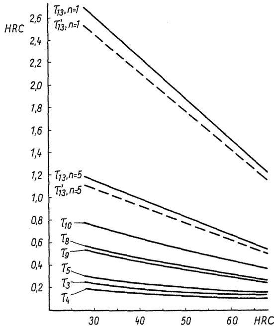
Fig. 7. 99% confidence limits of values obtained on various level hardness-measuring devices as a function of hardness.
