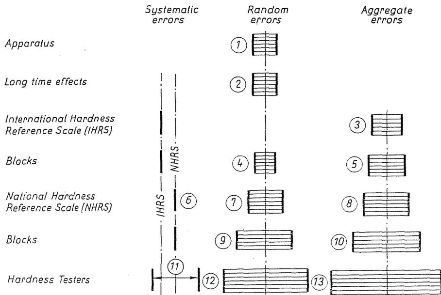
Fig. 3. Scheme of error propagation
