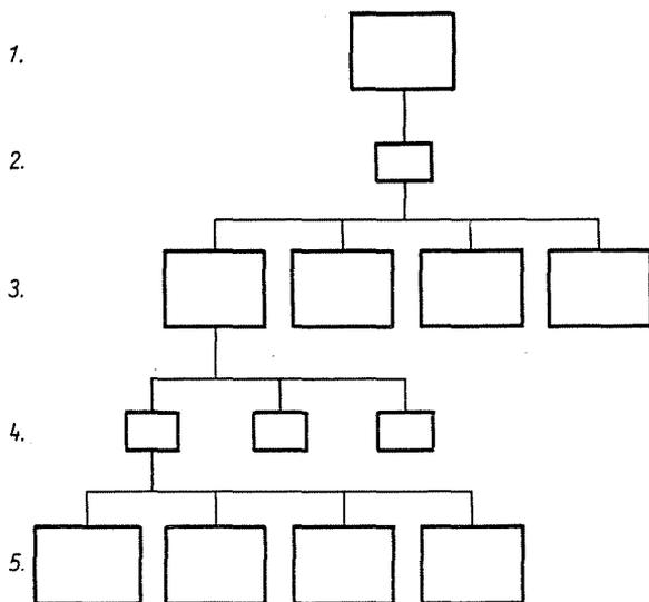
Fig. 2. Hierarchic order of hardness measurements according to a future international reference standard. 1 International hardness-reference standard-testing machine; 2 and 4 Hardness-reference blocks; 3 National hardness standard-testing machines; 5 Hardness testers in the industry
