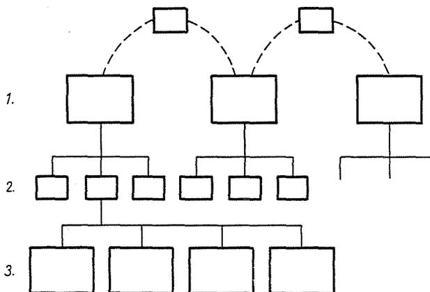
Fig. 1. Hierarchic order of hardness measurements. Present state. 1 National hardness-standard-testing machines; 2 Hardness reference blocks; 3 Hardness testers in the industry
